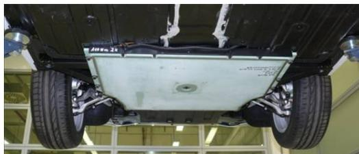
Figure 10: Secondary Coil after Vehicle Integration
