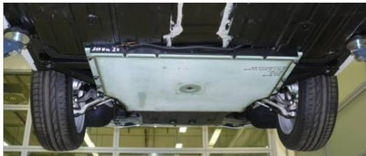
Figure 10: Secondary Coil after Vehicle Integration
