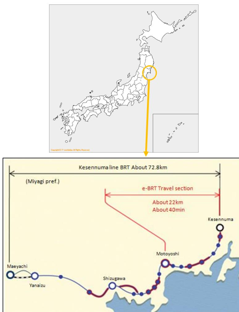
Figure 1: e-BRT operation section
