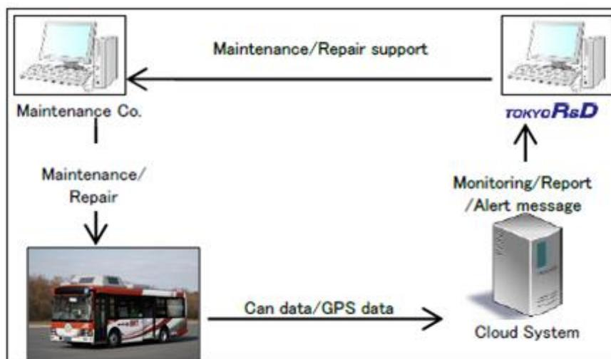
Figure 5: Maintenance system utilizing vehicle monitoring system
