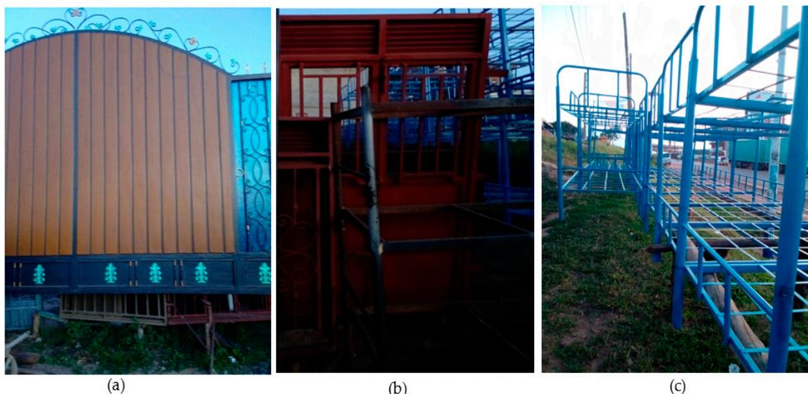
**Figure 2.** Some of the fabricated products at the metallic fabrication workshops considered in this study: (a) a security gate, (b) a metallic door and window, and (c) metallic double-decker beds.
