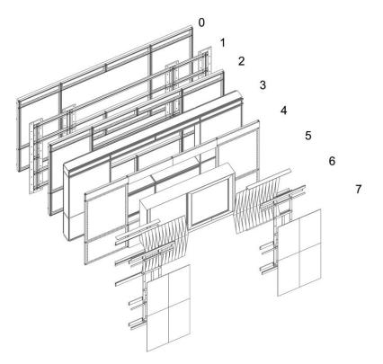
**Figure 11.** Isometric view of an exemplary façade component with axonometric illustration of the individual layers. The component layer numbers from 0 (inside) to 7 (outside) refer to the detailed description of the building envelope system in Table 6.
