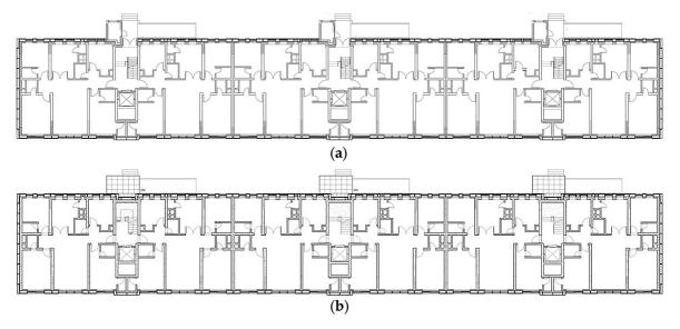
**Figure 16.** Reference first floor (**a**) and the second floor (**b**) plans of the renovated apartment building 103 with new building envelope and modified floor plan layouts.
