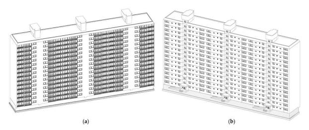
**Figure 4.** Isometric view from the South (**a**) and the North (**b**) of the virtual apartment building 103 model, reconstructed with the BIM software Revit.
