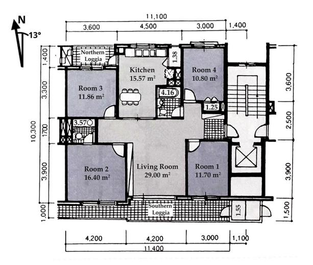
Figure 3. Typical floor plan of an apartment unit and rooms net floor area (in square meters) in the selected building 103 [25].
