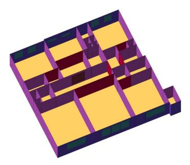
**Figure 13.** Isometric view of the Energyplus model of the renovated reference apartment unit with new room layout.
