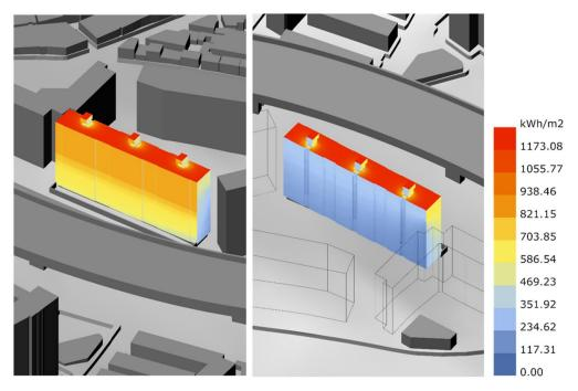
**Figure 7.** Isometric views from South-East (left) and North-West (right) of building 103 with global radiation received in kWh/a.
