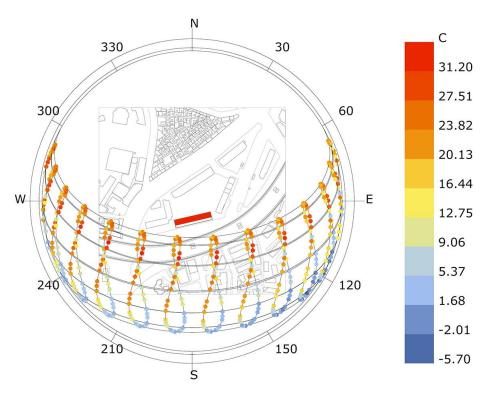
**Figure 6.** Sun path map with annual analysis and yearly dry-bulb temperature values associated to the position of the sun calculated for the 1st, 15th, 25th and last days of each month.
