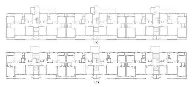
**Figure 5.** Ground floor (**a**) and second to 15 floor plans (**b**) of apartment building 103 reconstructed with the BIM software Revit.
