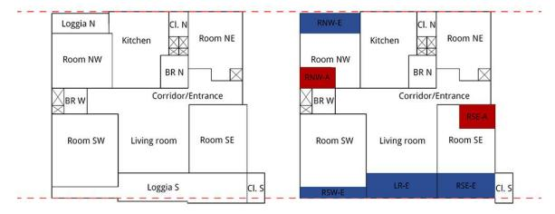
**Figure 10.** Reference apartment unit floor plan layouts before (left) and after (right) renovation. Loggia spaces that have been integrated in the adjacent rooms are marked blue. Additional storage rooms are marked red.
