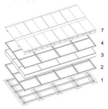
**Figure 12.** Isometric view of an exemplary roof component with axonometric illustration of the individual layers. The component layer numbers from 1 (inside) to 7 (outside) refer to the detailed description of the building envelope system in Table 6.
