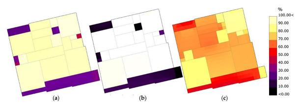
**Figure 9.** Reference apartment unit comfort maps on simplified floor plans with illustration of comfort hours' percentages in relation to all hours for different periods, (**a**) the period of one year; (**b**) winter and heating period from 1st January to 31st May; (**c**) summer and cooling period from 1st of June to 30th September.
