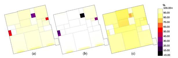
**Figure 14.** Floor plans with adaptive comfort maps of the renovated reference apartment unit illustrate (a) the annual amount of comfort hours, (b) the comfort hours from 1 January to 31 May and (c) the comfort hours from 1 June to 30 September. Comfort hours are illustrated in percentages of total hours from black (0%) to white (100%).
