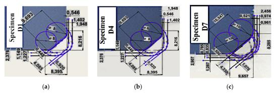
**Figure 4.** The macroscopic analysis: (**a**) For the specimen D1 without rehabilitation; (**b**) For specimen D4 by using the "grinding weld toe"; (**c**) For specimen D7 by using the "WIG re-melting weld toe."
