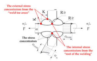
**Figure 1.** The "weld toe" areas, of the stress concentration; K-the cord of the welding seam; R/r the radius of the connection between the filler and the base material.
