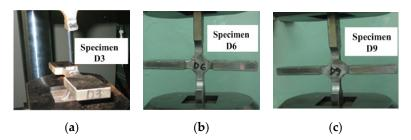
**Figure 9.** Fatigue tests: (**a**) For specimen D3without rehabilitation; (**b**) For specimen D6withby using the "grinding weld toe"; (**c**) For specimen D9 by using the "WIG re-melting weld toe."
