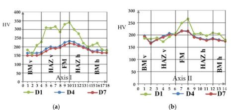
**Figure 7.** The variation of micro-hardness HV 0.1: (**a**) For specimens D1, D4 and D7 from axis I; (**b**) For specimen s D1, D4 and D7 from the axis II.
