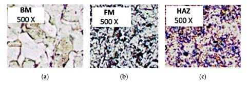
**Figure 5.** The microscopic analysis: (**a**) For specimen D1 without rehabilitation; (**b**) For the specimen D4 using the "grinding weld toe"; (**c**) For specimen D7 using the "WIG re-melting weld toe."
