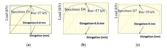
**Figure 10.** The stress-strain curves for the static tensile tests: (**a**) For specimen D1 without rehabilitation; (**b**) For specimen D4 by using the "grinding weld toe"; (**c**) For specimen D7 by using the "WIG re-melting weld toe."
