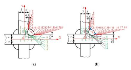
**Figure 6.** The measurements for micro-hardness HV 0.1: (**a**) For specimens D1 without rehabilitation and for D4 using the "grinding weld toe"; (**b**) For the specimen D7 using the "WIG re-melting weld toe."
