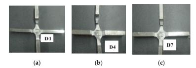
**Figure 8.** The static tensile tests: (**a**) For specimen D1without rehabilitation; (**b**) For specimen D4by using the "grinding weld toe"; (**c**) For specimen D7 by using the "WIG re-melting weld toe."
