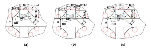
**Figure 3.** The cross sections of the specimens: (a) Specimens D1, D2, D3 without rehabilitation; (b) Specimens D4, D5, D6 by using the "grinding weld toe" rehabilitation technique; (c) Specimens D7, D8, D9 by using the "WIG re-melting weld toe" rehabilitation technique.
