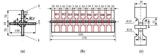
**Figure 2.** The shape and size of the welding sample D, expressed in millimetres; (**a**) front view sketch welding sample, (**b**) test specimens from D1-D9, (**c**) static and fatigue specimen tests after milling.
