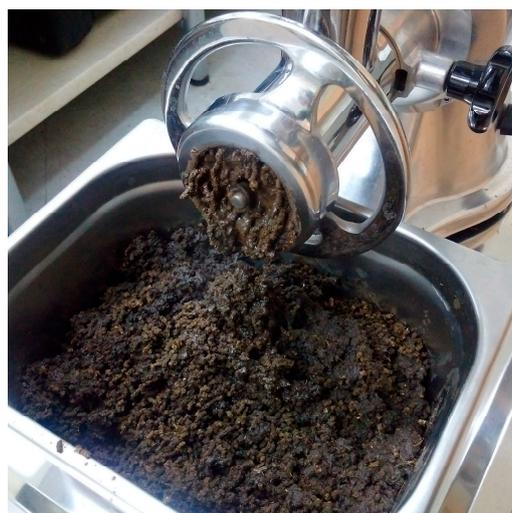
**Figure 3.** Solid fraction of digestate fragmented to 3 mm—granules component.
