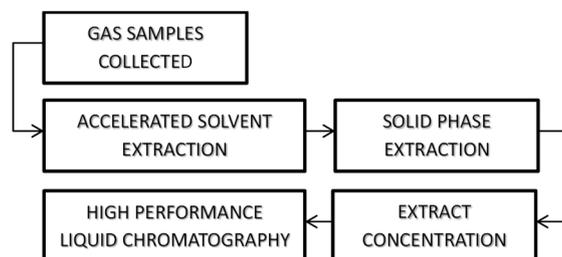
**Figure 2.** Schematic diagram of analytical procedure.
