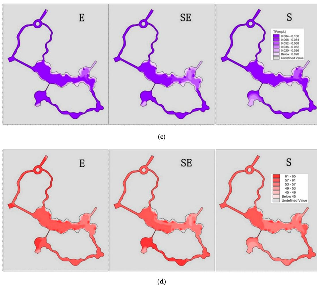
**Figure 10.** Chl-a distribution (a), TN distribution (b), TP distribution (c) and comprehensive score of eutrophication assessment (d) with no water diversion under different wind conditions.
