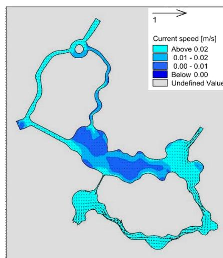
**Figure 9.** Flow field with water diversion through sluice.
