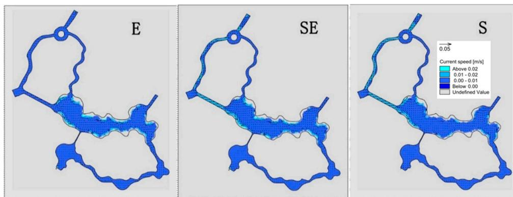
**Figure 7.** Velocity distribution in different wind directions without water diversion.
