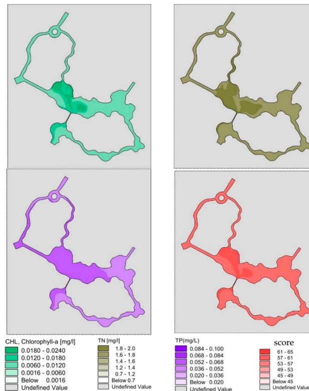
**Figure 12.** Chl-a, TN and TP concentrations and eutrophication comprehensive score with water diversion through sluice.
