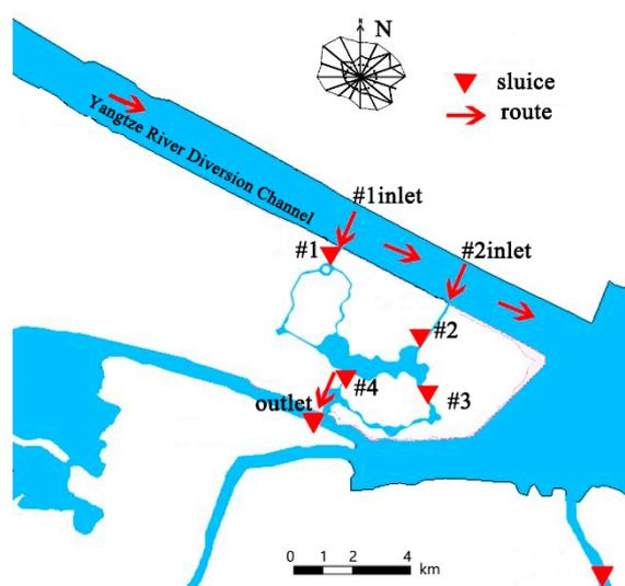
**Figure 5.** Route of water diversion through three sluices (#1-3) and one culvert (#4).
