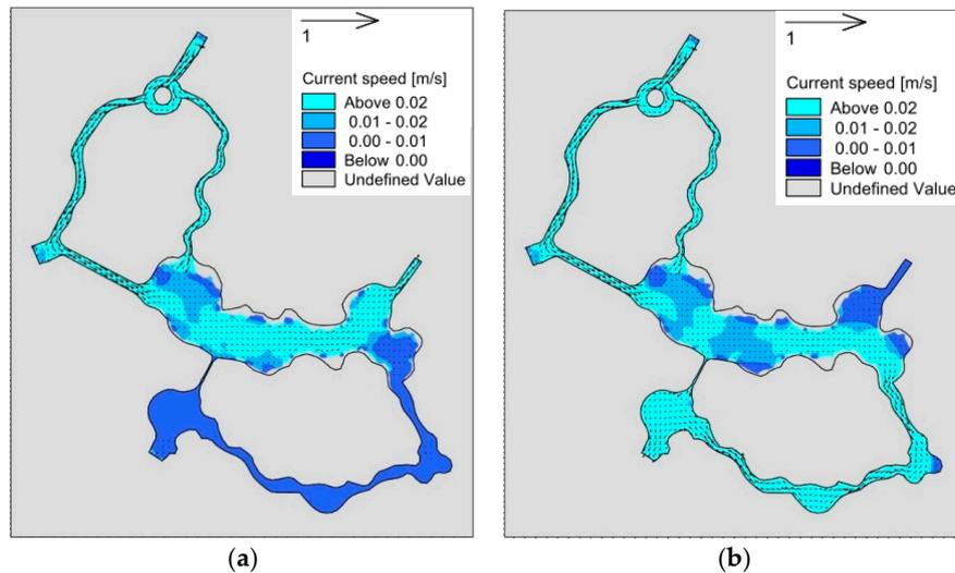
**Figure 8.** (a) Flow field with water diversion through pump for 22 h. (b) Flow field with water diversion through pump for 30 h.
