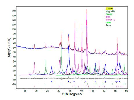
Figure 1. XRD analysis of ultrafine fly ash.
