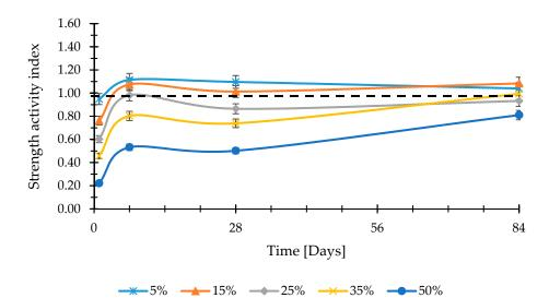
Figure 9. Strength activity index of mortars manufactured with CEM II/A-LL and FA.
