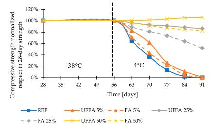
**Figure 17.** Compressive strength over time normalized respect to 28-day compressive strength of specimens stored in 30 wt % CaCl<sub>2</sub> solution.
