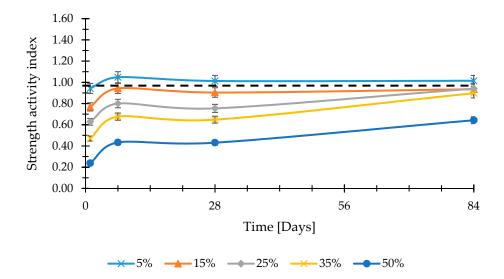
Figure 11. Strength activity index of mortars manufactured with CEM III/A and FA.
