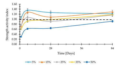
Figure 8. Strength activity index of mortars manufactured with CEM II/A-LL and UFFA.
