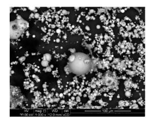
Figure 3. SEM image of fly ash.
