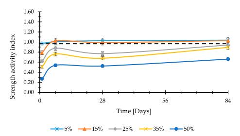
Figure 7. Strength activity index of mortars manufactured with CEM I and FA.
