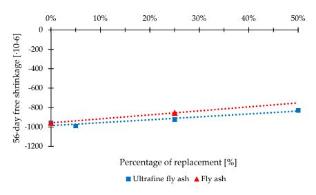
Figure 16. Free shrinkage after 56 days of mortars vs. percentage of replacement.
