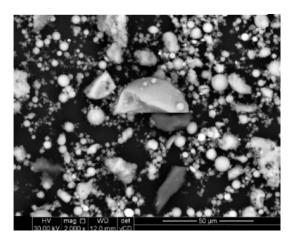
Figure 2. SEM image of ultrafine fly ash.
