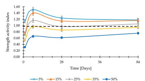
Figure 12. Strength activity index of mortars manufactured with CEM III/B and UFFA.
