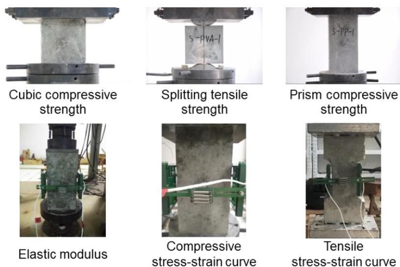
Figure 4. Mechanical property test setups.
