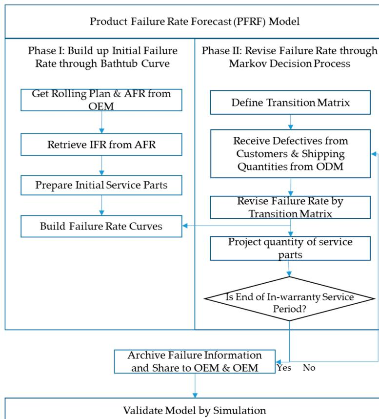
**Figure 4.** The Product Failure Rate Forecasting (PFRF) Model.
