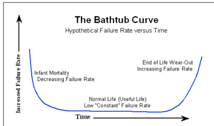
**Figure 2.** A Typical Life Cycle Bathtub Curve (Sourced from “Reliability and MTBF Overview”, Victor Reliability Engineering).
