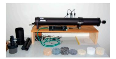
Figure 4. Kundt impedance tube Type 4206 and STERED<sup>®</sup> samples.
