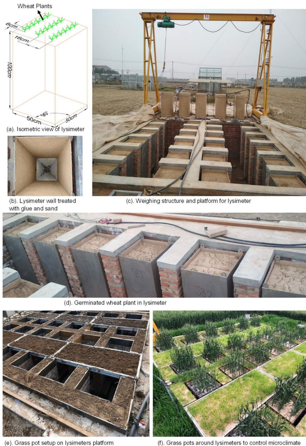
Figure 2. Schematic descriptions of the experimental device. (a) Isometric view of lysimeters (plant seed location); (b) Lysimeter wall treated with glue and sand; (c) Weighing structure and platform for lysimeters; (d) Germinated wheat plant in lysimeters; (e) Grass pot set up on lysimeters platform; (f) Grass pots around lysimeters to control microclimate.
