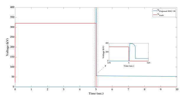
Figure 8. The CB voltage and voltage at the fault location after applying a short-circuit DC fault at 5 s.
