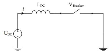
Figure 5. Equivalent circuit of the DC CB in the DC grid.
