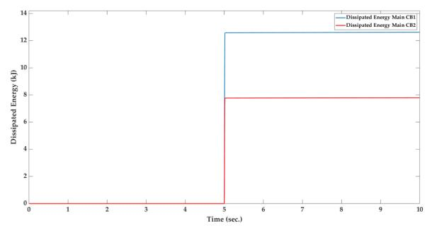
**Figure 9.** The dissipated energy of the surge arrestors in the two main DC CBs of the proposed HDCCB after applying a short-circuit DC fault at 5 s.
