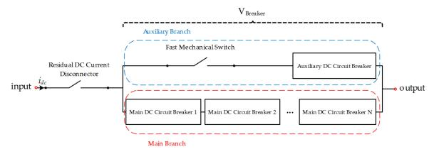
Figure 1. Overall structure of the proposed HDCCB.
