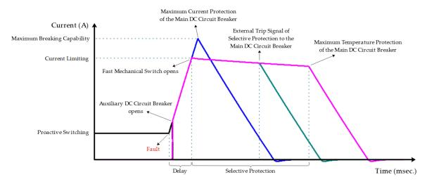
Figure 4. The current waveform of a typical proactive HDCCB.
