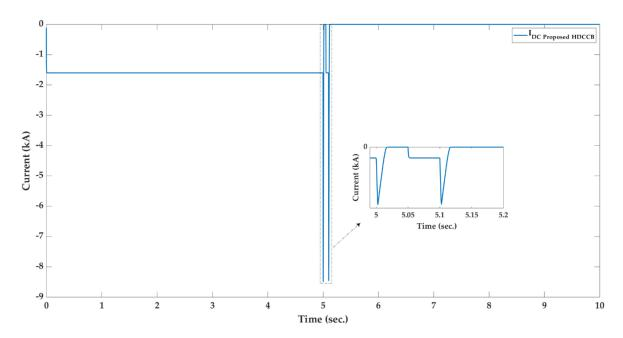
**Figure 14.** The DC current of the proposed HDCCB in reclosing and rebreaking tests in the reverse current interruption.
