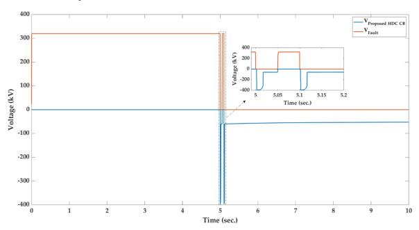
**Figure 15.** The CB voltage and voltage at the fault location in reclosing and rebreaking test in the reverse current interruption.
