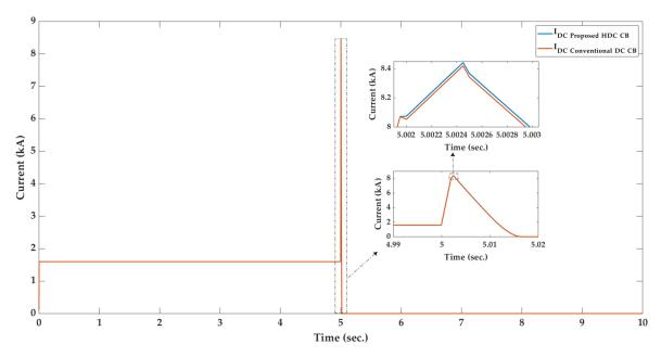
**Figure 17.** Comparison between the DC current response of the proposed HDCCB and the conventional DC CB after applying a short-circuit DC fault at 5 s.
