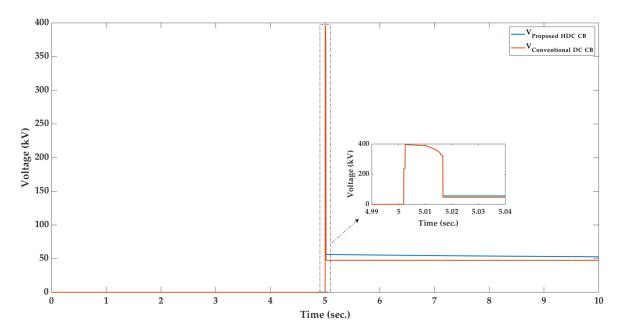
**Figure 16.** Comparison between the voltage response of the proposed HDCCB and the conventional DC CB after applying a short-circuit DC fault at 5 s.
