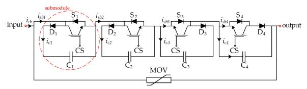
Figure 2. Configuration of the main DC CBs in the main branch.
