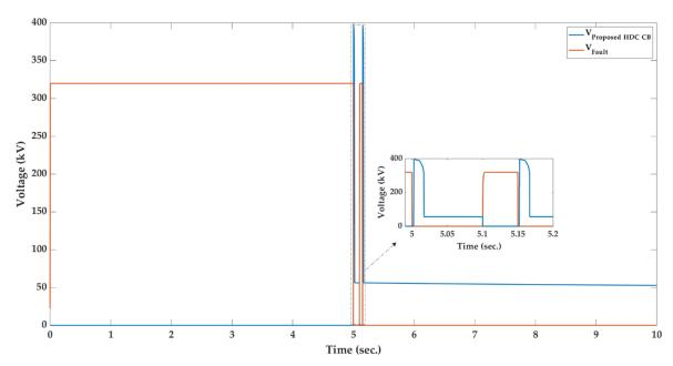
**Figure 13.** The CB voltage and voltage at the fault location in reclosing and rebreaking test in the rated current interruption.
