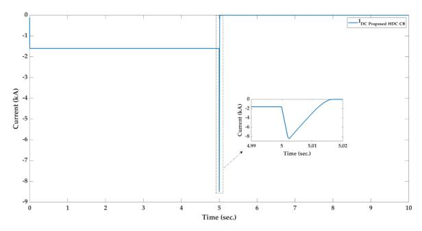
**Figure 10.** The DC current of the proposed HDCCB after applying a short-circuit DC fault at 5 s after changing the direction of the proposed HDCCB.
