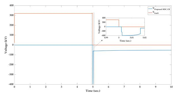
**Figure 11.** The CB voltage and voltage at the fault location after applying a short-circuit DC fault at 5 s after changing the direction of the proposed HDCCB.
