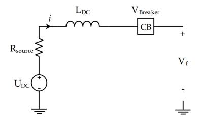
Figure 6. Configuration of the DC-link for fault analysis.
