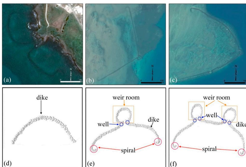
**Figure 4.** Upper panel shows GE images for three typical stone tidal weirs (STWs), including (a) arched, (b) single-room, and (c) double-room STWs. The lower panel shows schematic views corresponding to the GE images on the upper.
