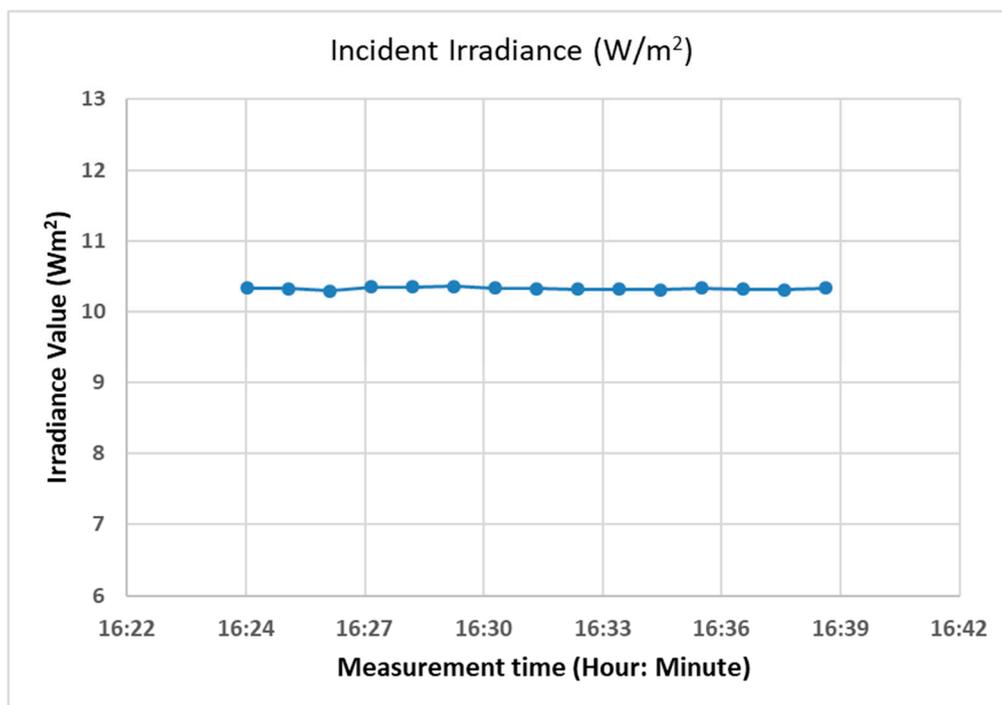
Figure 5. Measured incident irradiance during the electrical characterizations and measurements.
