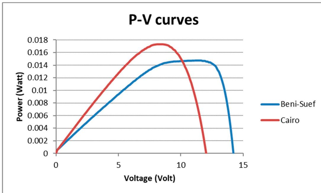
Figure 4. P–V (Power–Voltage) curves of the tested PV modules.
