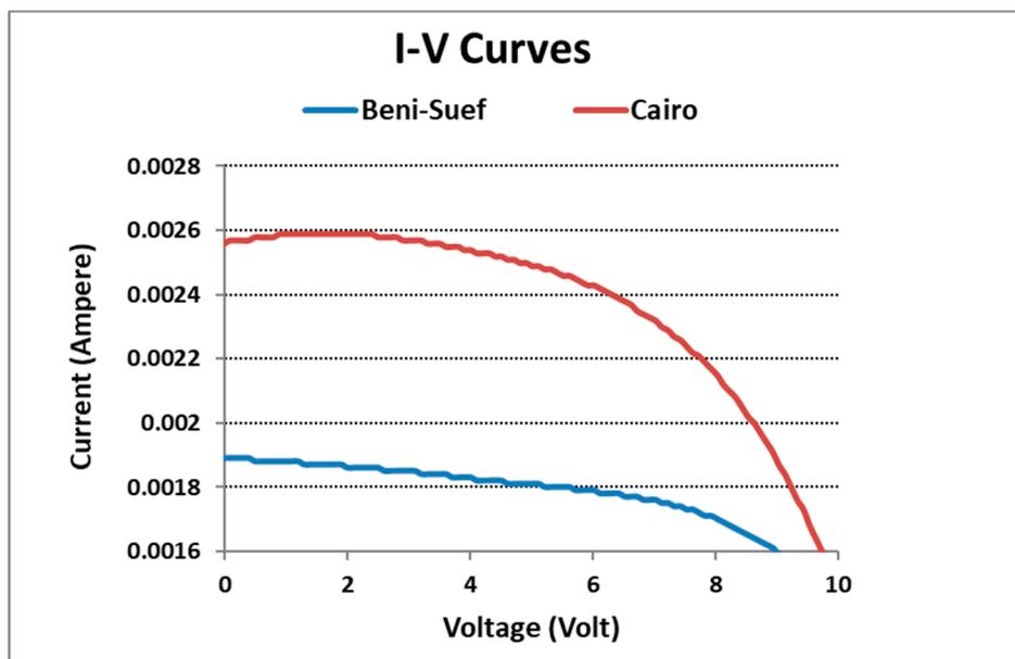
Figure 3. IV (Current–Voltage) curves of the tested PV modules.
