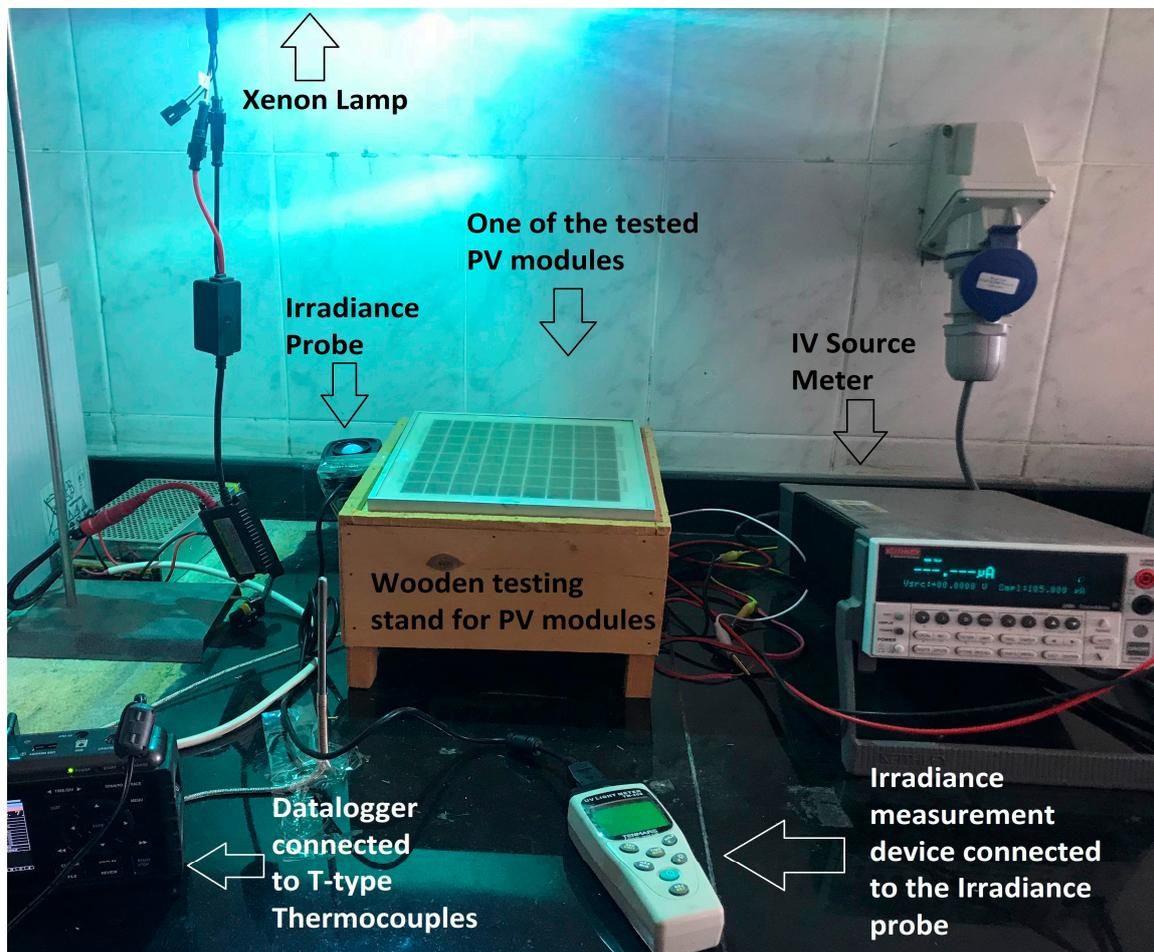
**Figure 1.** The indoor testing station for the PV modules.
