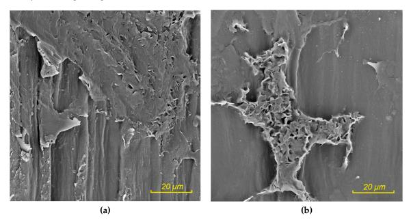
**Figure 10.** Particle board from rapeseed straw bonded with UF adhesive, enzymatically treated (combination) rapeseed particles; (**a**) adhesion and cohesion error, (**b**) failure in the pith of the particles.
