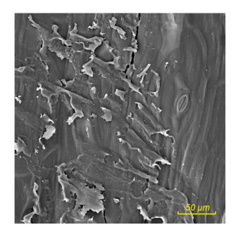
**Figure 11.** Particle board from rapeseed straw bonded with UF adhesive, enzymatically treated (xylanases) rapeseed particles; adhesion error.
