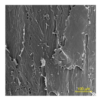
**Figure 7.** Particle board made of wheat straw bonded with UF adhesive, enzymatically treated (xylanases) wheat particles; adhesion failure.
