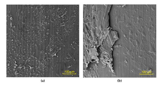
**Figure 15.** Particle board from wheat husks bonded with UF adhesive, untreated husks; (**a**) poor spilling of the adhesive, (**b**) impurities in the adhesive.
