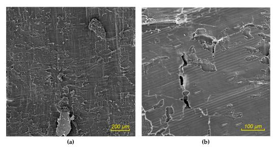
**Figure 14.** Particle board from wheat straw bonded with UF adhesive, plasma treated particles, higher degree of treatment; (**a**) adhesion and cohesion failure in the adhesive, (**b**) adhesion error.
