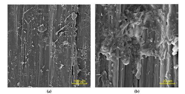
**Figure 13.** Particle board from wheat straw bonded with UF adhesive, plasma treated particles, weaker degree of treatment; (**a**) adhesion and cohesion failure, (**b**) dust particles in the adhesive.
