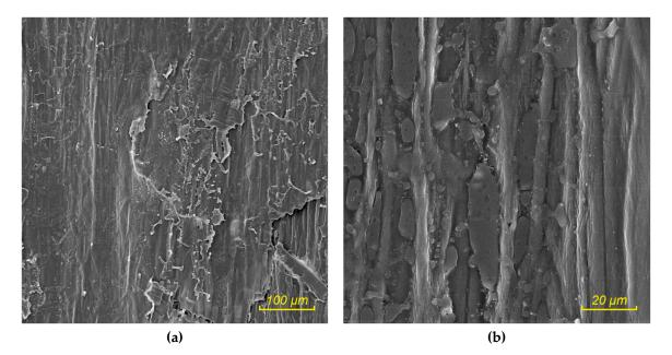
**Figure 6.** Particle board made of wheat straw bonded with UF adhesive, enzymatically treated (combination) wheat particles; (**a**) mixed character of joint failure, (**b**) bubbles in the adhesive.
