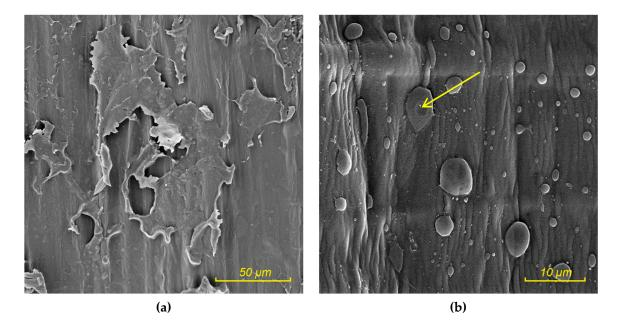
**Figure 9.** Particle board from rapeseed straw bonded with UF adhesive, enzymatically treated (xylanases) rapeseed particles; (**a**) adhesion error, (**b**) bubbles in the adhesive.
