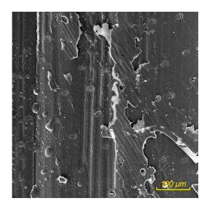
**Figure 16.** Particle board from wheat husks bonded with UF adhesive, hydrothermally treated husks; nature of the spilling of the adhesive on the surface of the husks.
