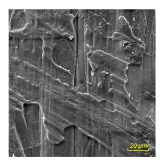
**Figure 5.** Particle board made of wheat straw bonded with UF adhesive, enzymatically (pectinases) treated wheat particles; adhesion error.
