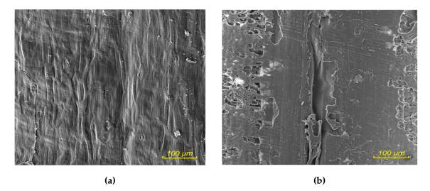
**Figure 4.** Particle board made of wheat straw bonded with urea-formaldehyde adhesive (UF) adhesive, untreated wheat particles; (**a**) adhesion error-particle, (**b**) adhesion error-adhesive.
