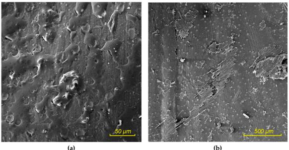
or partially spilled drops. Larger peel layers with an impression of the torn-off material are often visible (Figure 18b). The disadvantage of the dry treatment is the higher incidence of impurities.
