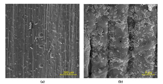
**Figure 17.** Particle board from wheat husks bonded with UF adhesive, alkaline treated husks; (a) dispersion of adhesive, (b) NaOH residues on the surface of husks.
