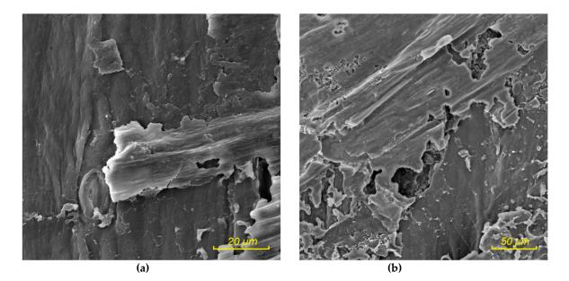
**Figure 1.** Particle board from rapeseed straw bonded with epoxy-polyester adhesive, untreated particles; (**a**) thorough spill of adhesive on the surface of the particles, (**b**) adhesion error.
