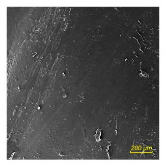
**Figure 12.** Particle board from wheat straw bonded with UF adhesive, plasma untreated particles; adhesion error.
