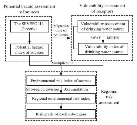
**Figure 2.** A coupling model for environmental risk assessment of accidental pollution incidents in a drinking water source area.
