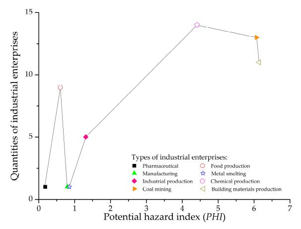
Figure 4. The cumulative potential hazard index of different types of hazardous industrial enterprises.
