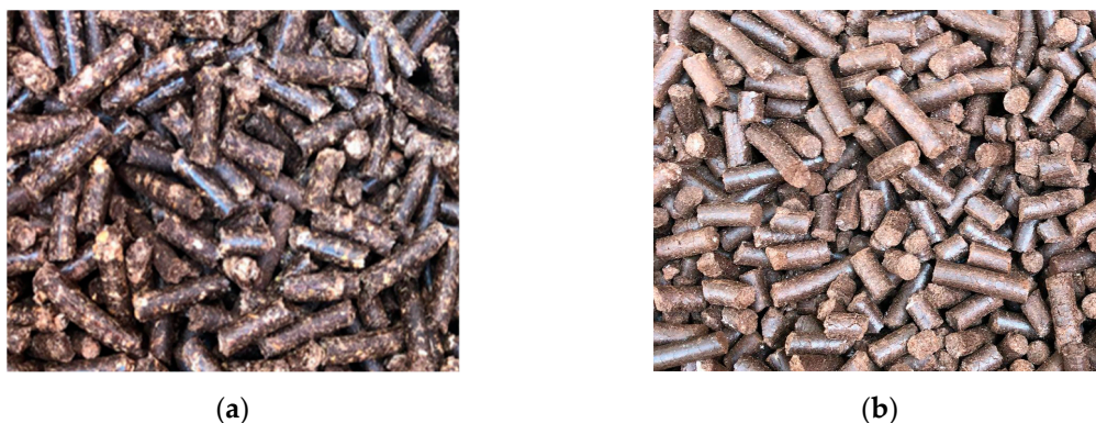
Figure 4. (a) Spent coffee grounds (SCG) (50%) and pine sawdust (50%) pellet; (b) SCG (98%) and corn starch (2%) pellet.
