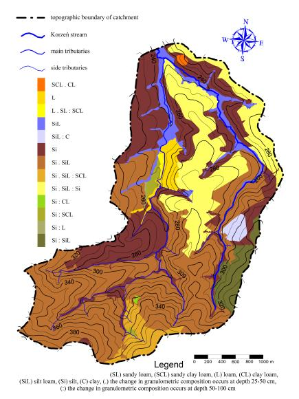
Figure 5. Soil distribution map of the flysh stream in catchment area.
