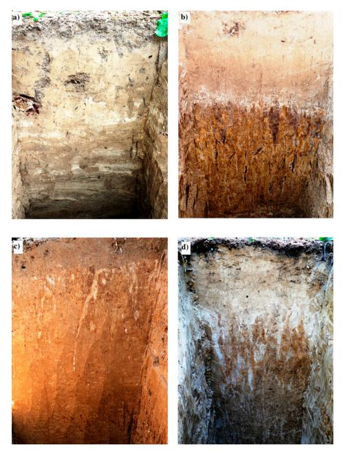
**Figure 4.** Soil profiles in the studied catchment: (**a**) Stagnic Cambisol, (**b**) Stagnic Luvisol, (**c**) Hamplic Cambisol, and (**d**) Albic Podzol.
