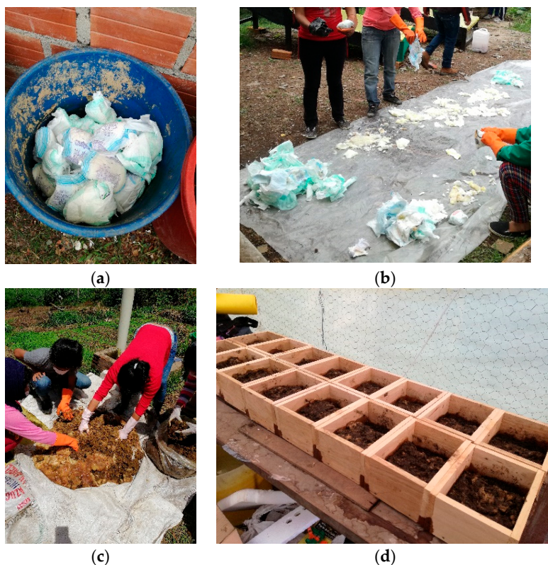
Figure 3. Photos of the experimental procedure: (a) collection of the used baby diapers (UBDs); (b) preparation of the substrate for the treatment; (c) mixing with cow dung, earthworms, and AB; (d) location in wooden boxes.
