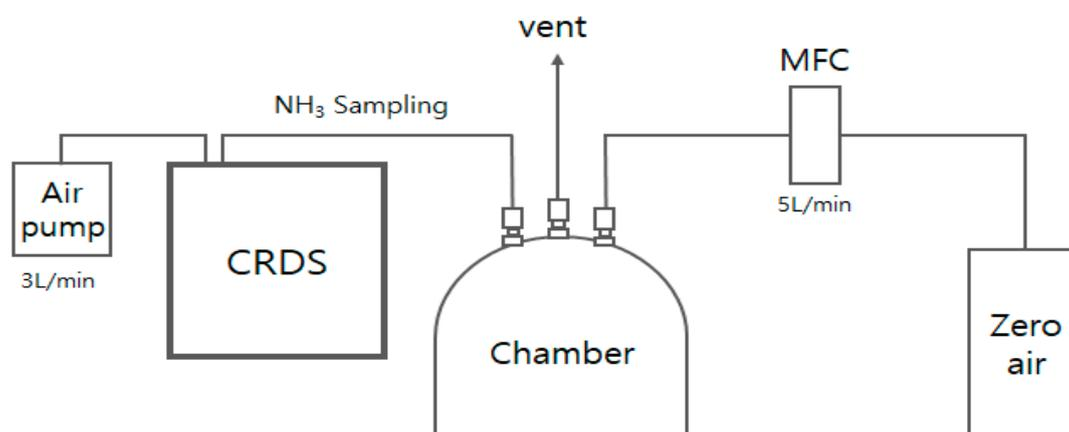
**Figure 2.** Schematic of the field setup using the cavity ring-down spectrometer (CRDS).
