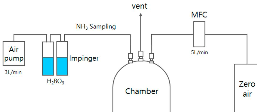
**Figure 3.** Schematic of the field setup using the indophenol method.
