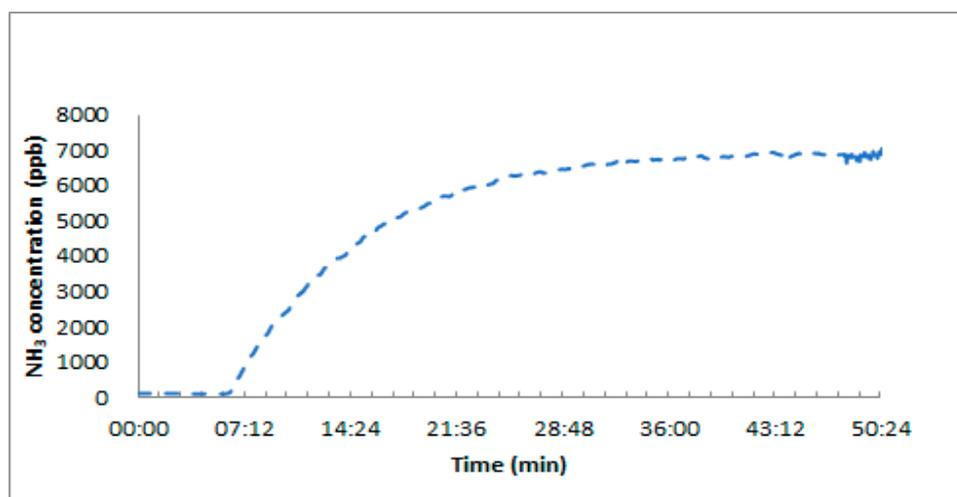
Figure 9. Ammonia concentration in an open chamber according to a field sample.
