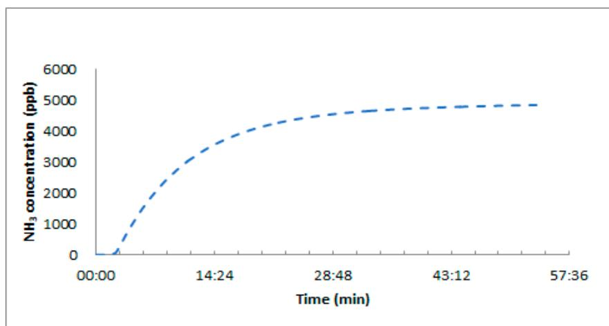
**Figure 5.** Stabilization time of ammonia concentration in the chamber according to STD (standard gas) 5 ppm.
