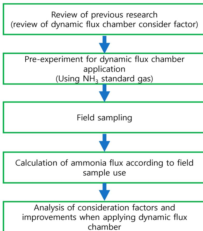
**Figure 1.** Process of research procedure for applying a dynamic flux chamber in a barn.
