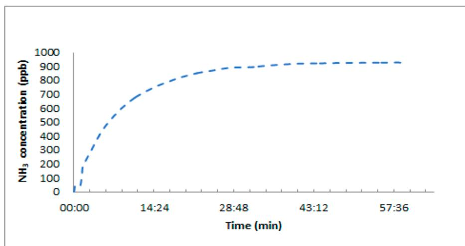
**Figure 6.** Stabilization time of ammonia concentration in the chamber according to STD 1 ppm.
