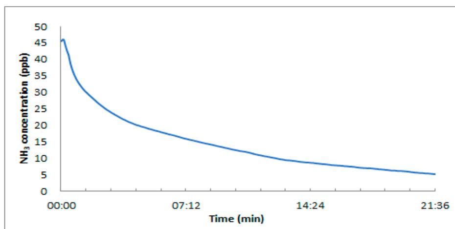
**Figure 4.** Stabilization time of ammonia concentration according to zero air input.
