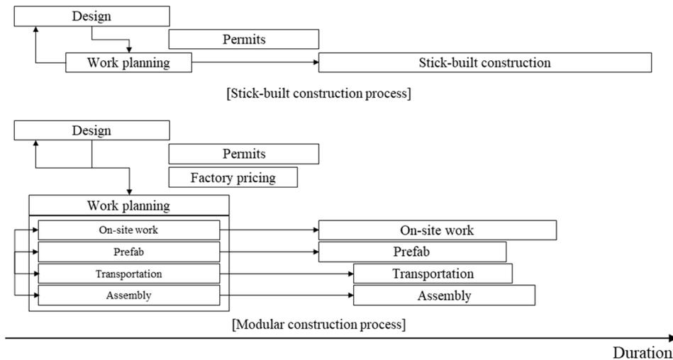
Figure 1. Increased complexity caused by interposed processes.
