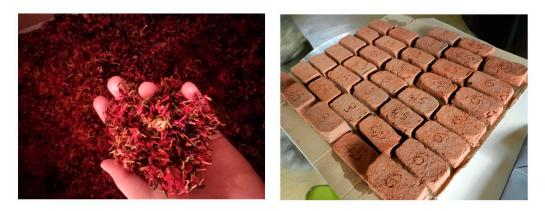
**Figure 2.** MAST (Mattone in Argilla con Scarti Tessili—Clay Brick from Textile Waste): from textile waste to experimental specimens. On the left, shredded polyester threads; on the right, clay bricks obtained with different percentages of polyester waste.
