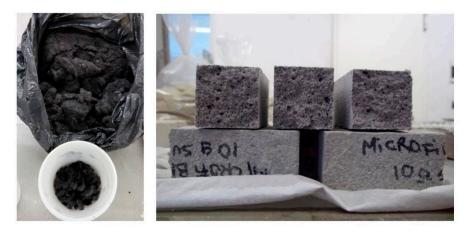
**Figure 3.** ReCash Plaster (Recycled Cashmere for Plaster): from textile waste to experimental specimens. On the left, wool and cashmere dust; on the right, pre-mixed plaster obtained by replacing glass fibres with textile waste.
