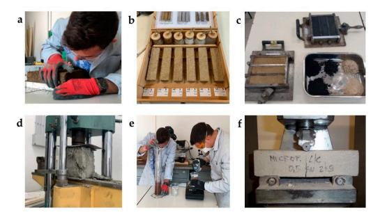
**Figure 1.** Experimental activities at the LaSTIn laboratory (Politecnico di Torino) on different materials, for example: (**a**) manufacture of a concrete and hazelnut shell specimen; (**b**) manufacture of specimens using rice husks and natural adhesives; (**c**) shaping of specimens using hemp and biochar; (**d**) compression test of a concrete and natural fibre specimen; (**e**) weighing and mixing of agri-food waste; (**f**) flexure test of a plaster specimen using textile waste.
