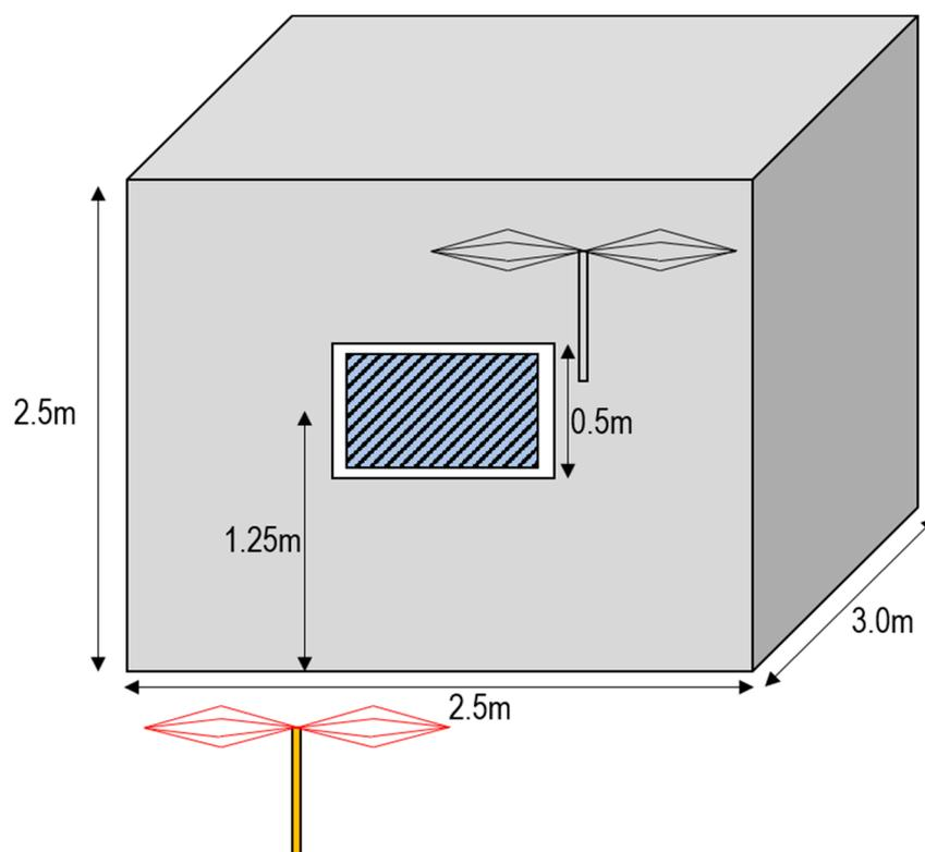
**Figure 5.** SE test setup.
