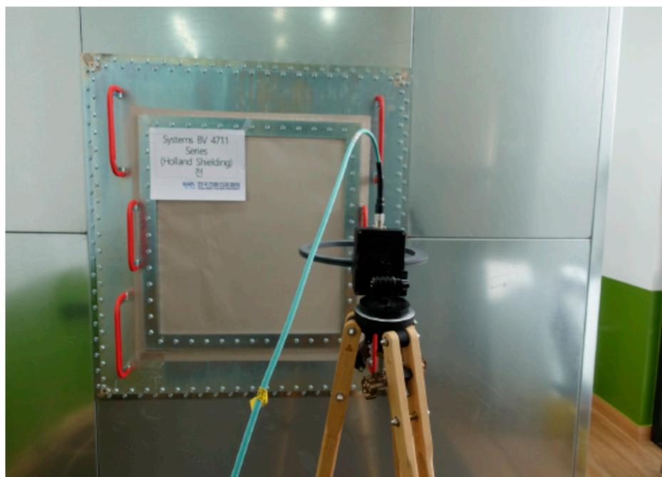
Figure 6. SE test setup.
