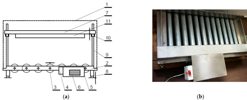
**Figure 1.** Stand for potato tubers UV-C radiation: (a) stand layout, (b) view of rotating rollers. L: 1: chamber housing, 2: device frame, 3: rotating rollers, 4: mechanism for gradeless regulation of roller rotation speed with the device switch, 5: engine, 6: engine cooling system, 7: radiator frame, 8: height-adjustable foot (screw mechanism for leveling the device), 9: radiator frame guide, 10: gradeless UV-C radiator control above the bottom of the chamber (rollers), 11: UV-C radiators.
