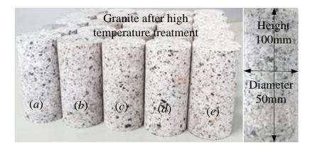
**Figure 1.** Granite samples after high-temperature treatment. (a) Temperature for room temperature,  $25 \degree C$ ; (b) Temperature for  $200 \degree C$ ; (c) Temperature for  $400 \degree C$ ; (d) Temperature for  $600 \degree C$ ; (e) Temperature for  $800 \degree C$ .
