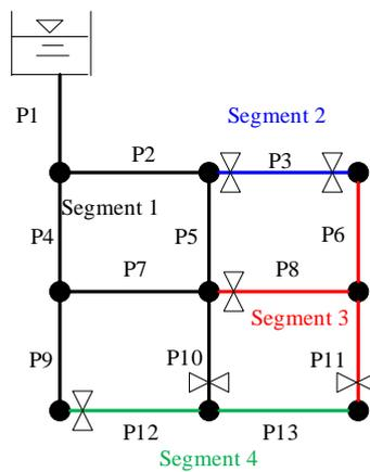
Figure 7. Illustration of segments formed by valves.
