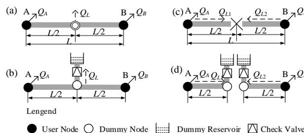
Figure 8. The hydraulic model of leak and break. (a) Illustration of the pipe leak, (b) Hydraulic model for pipe leak, (c) Illustration of the pipe break, (d) Hydraulic model for pipe break.
