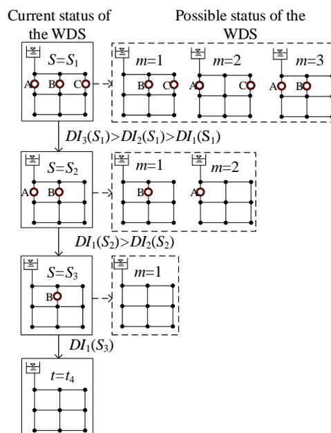
Figure 3. Illustration of the cost-benefit method schematic.
