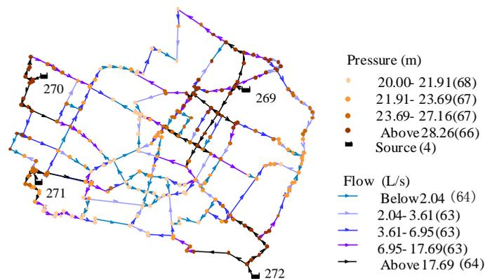
Figure 9. The water distribution network of Modena.
