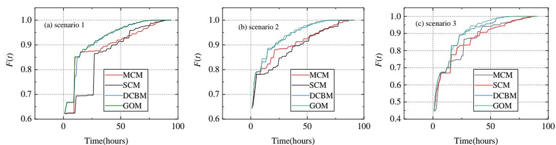
Figure 16. Restoration curves considering the positions of valves. (a) Scenario 1, (b) Scenario 2, (c) Scenario 3.
