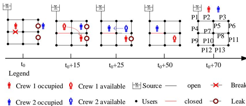
Figure 5. An example of the post-earthquake restoration process of WDS.
