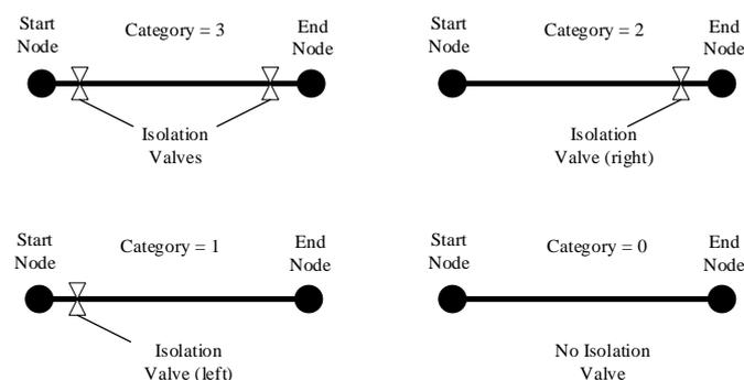
Figure 6. Pipeline categories according to the valve’s position.
