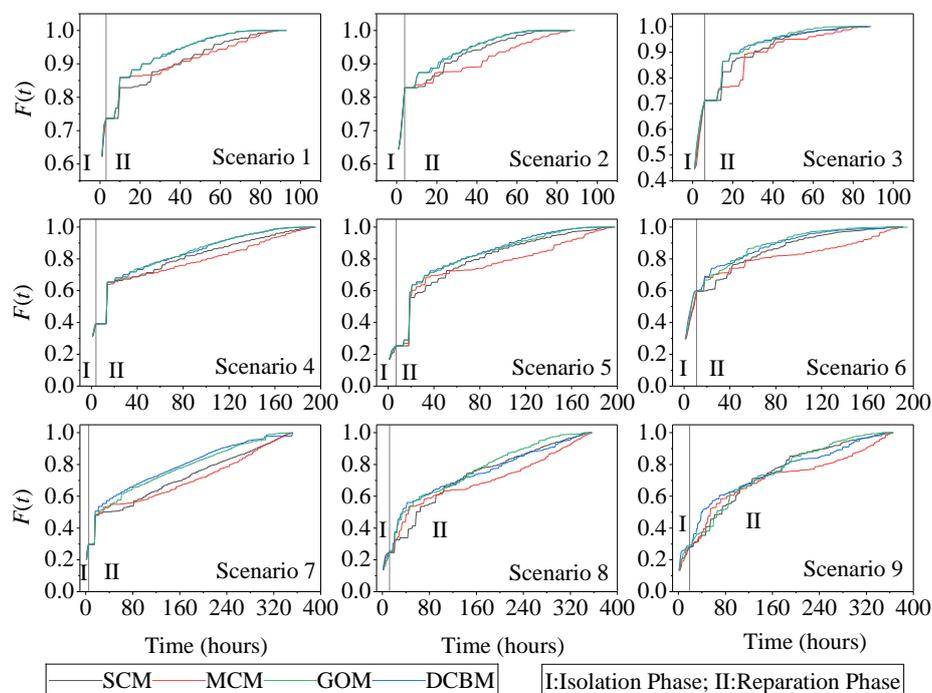
**Figure 11.** The functionality recovery curve for nine scenarios.
