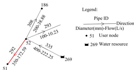
**Figure 13.** The partial network around resource 269.
