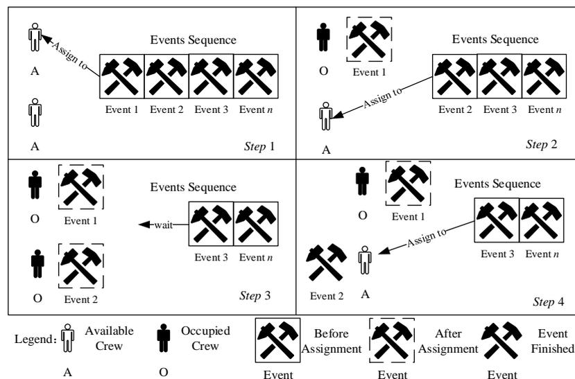
Figure 4. The procedure of the events assigned to the crews.
