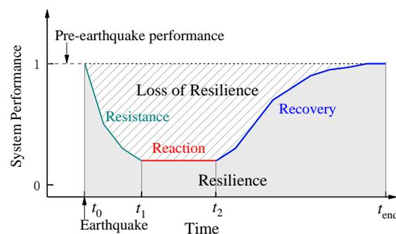
**Figure 1.** Performance curve of a water distribution system (WDS) following an earthquake.
