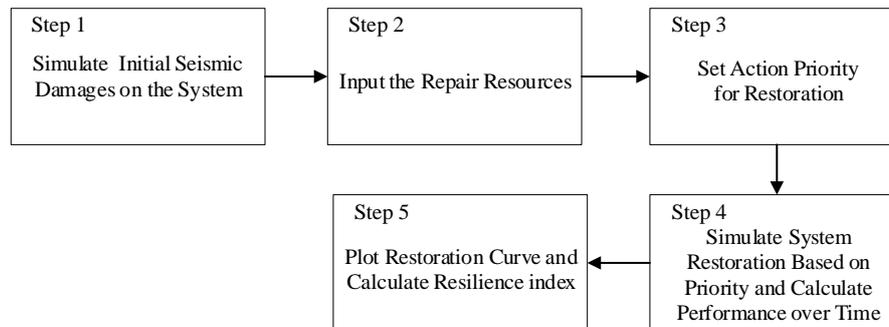
**Figure 2.** Flow chart of the framework for seismic resilience evaluation.
