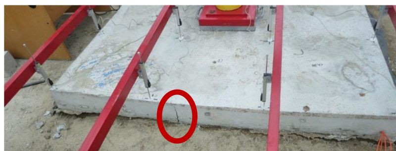
Figure 17. Vertical crack on slab G01; load 150 kN.
