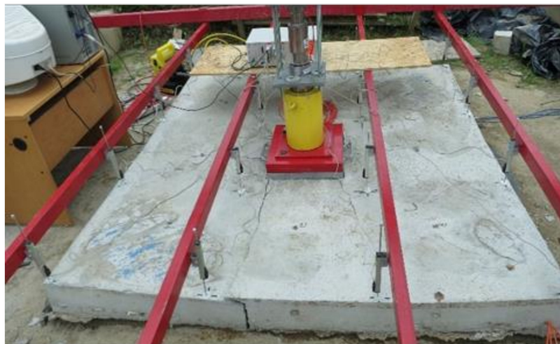
Figure 9. Load test of slab G01 on subsoil–slab failure.
