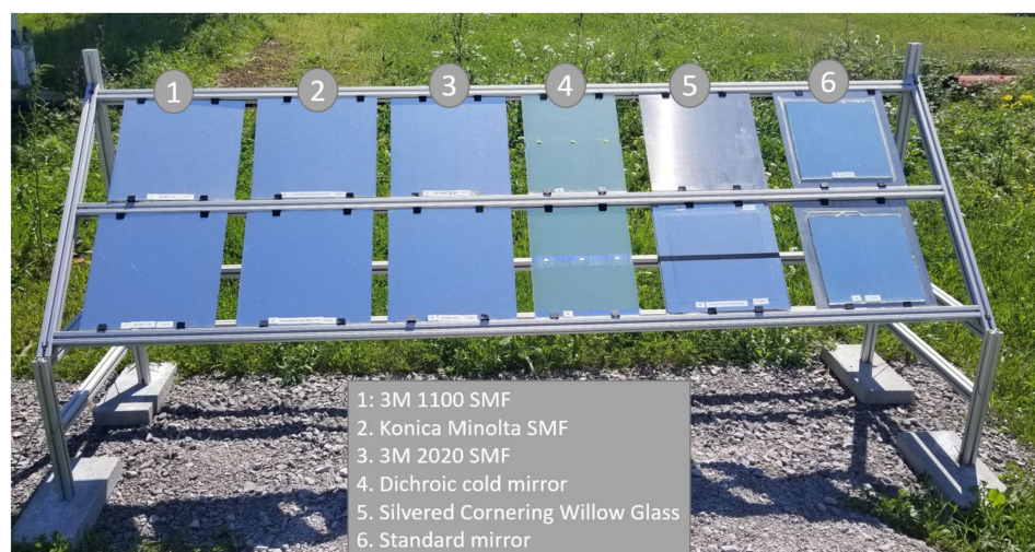
Figure 3. Concentrating solar panel reflector testbed installed at the Solar Applied Research and Testing (START) Lab in Crowley, Louisiana. Bottom row is cleaned for testing and the top is left dirty.
