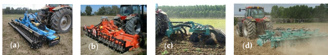
Figure 1. Selected implements during the tests. (a) 5 m power harrow; (b) 5.2 m rotary tiller; (c) combined cultivator; (d) offset disk harrow.
