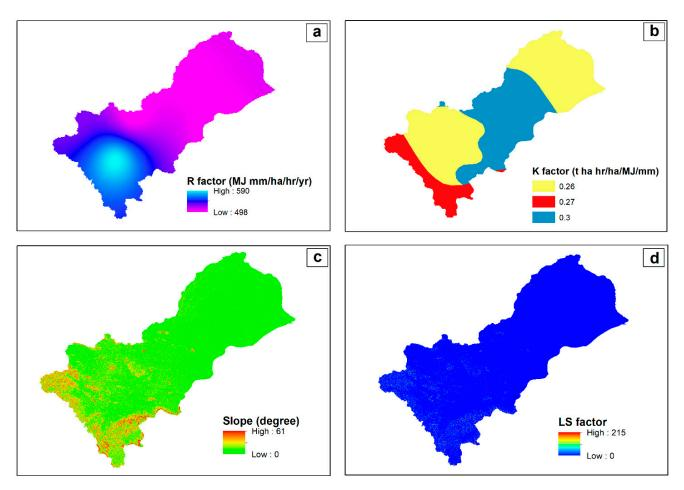
Figure 5. Maps of R-factor (a), K-factor (b), slope (c) and LS-factor (d) of the Sangkae catchment.
