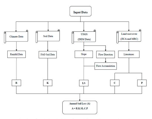
Figure 4. Flowchart of applied methodology for modelling soil erosion in the catchment.
