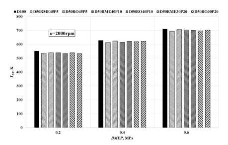
**Figure 7.** Comparison of  $T_{EX}$  of different fuel mixtures.
