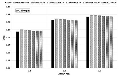
Figure 6. Comparison of *BTE* of different fuel mixtures.
