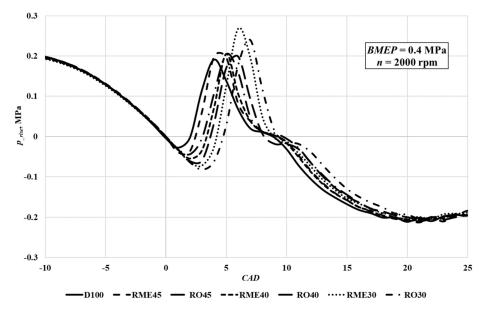
Figure 4. Comparison of *p* rise of different fuel mixtures.
