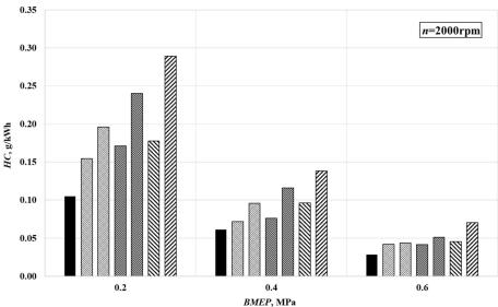
Figure 11. Comparison of HC of different fuel mixtures.
