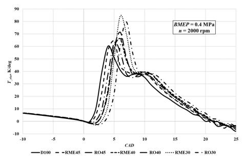
**Figure 3.** Comparison of *T*\_*rise* of different fuel mixtures.
