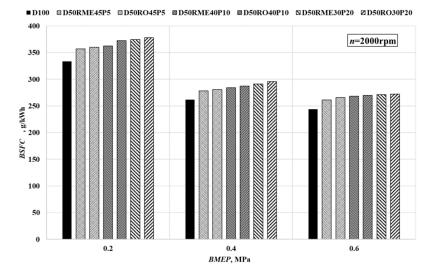
Figure 5. Comparison of BSFC of different fuel mixtures.
