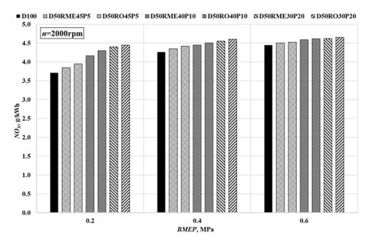
**Figure 12.** Comparison of  $NO_x$  of different fuel mixtures.
