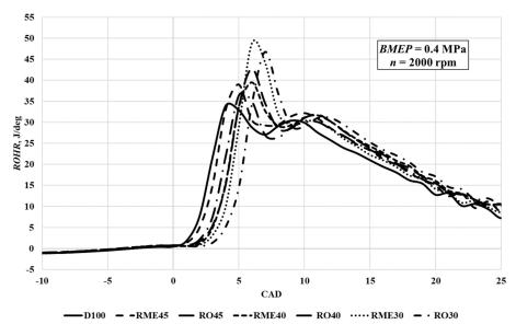
Figure 2. Comparison of ROHR of different fuel mixtures.
