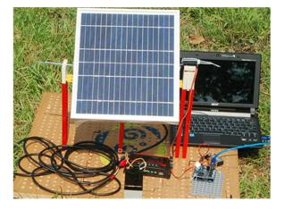
**Figure 7.** Students measured the angle between the solar panel and the sun, using Arduino control to obtain the best storage value ( $S_A$ - $A_3$ - $Y_6$ ).
