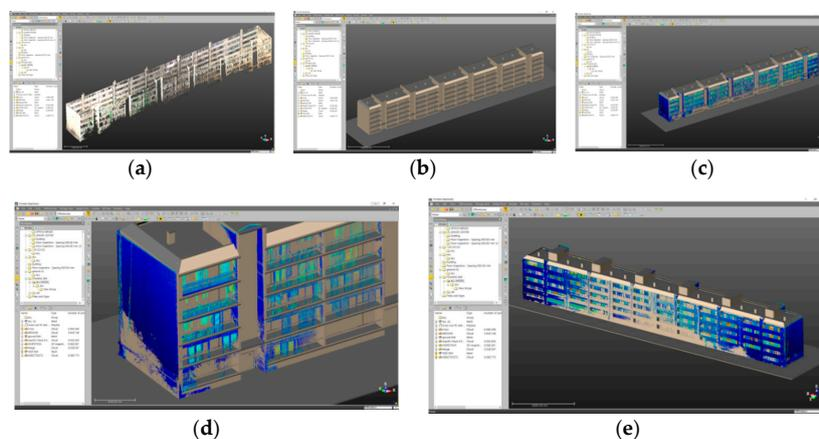
**Figure 6.** Combination of the point cloud and Building Information Modeling (BIM) data for existing drawings of Building E. (a) Point cloud data for Building E; (b) BIM data for Building E; (c) Data combination; (d) Point cloud data combined with BIM data; (e) Point cloud data combined with BIM data.
