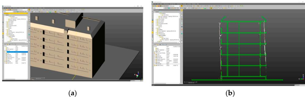
**Figure 10.** Analysis of Building E's slope. (a) Extraction of cross-sectional information from BIM data; (b) Results of examining Building E's overall slope.
