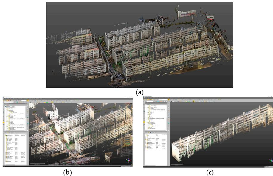
**Figure 5.** Analysis using only 3D scanning data. (a) Point cloud data for the Daeseong Apartment Complex; (b) Acquisition of point cloud data; (c) Extraction of Building E data.
