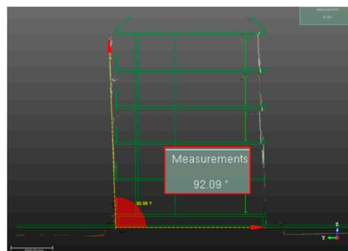
**Figure 11.** Slope analysis results for Building E.
