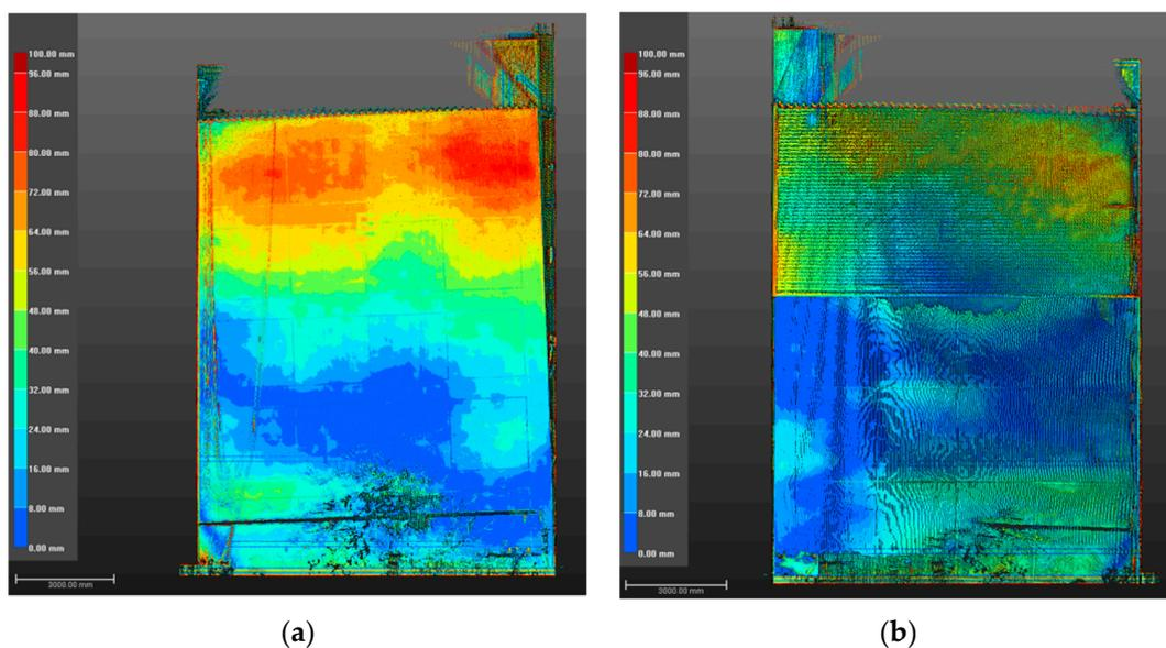
Figure 9. Smoothness analysis results for Building E's east and west walls. (a) Analysis of Building E's west wall; (b) Analysis of Building E's east wall.
