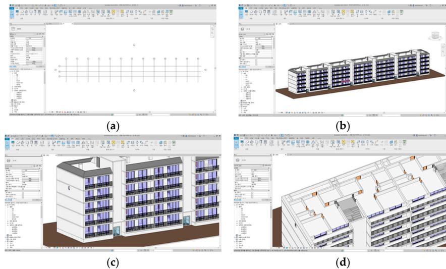
**Figure 3.** BIM modeling of the Daeseong Apartment Complex through reverse engineering of 3D geometry. (a) Grid setting for the BIM modeling of Building E; (b) BIM modeling of Building E; (c) Elevation of Building E; (d) Sectional view of Building E.
