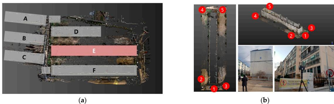
**Figure 4.** Field design for scanning the Daeseong Apartment Complex. (a) Location of Building E in the Daeseong Apartment Complex. A–F is the number of buildings in apartments; (b) Scanning measurement locations and on-site analysis. ①–⑤ is measurement points of the 3D scanner in on-site.
