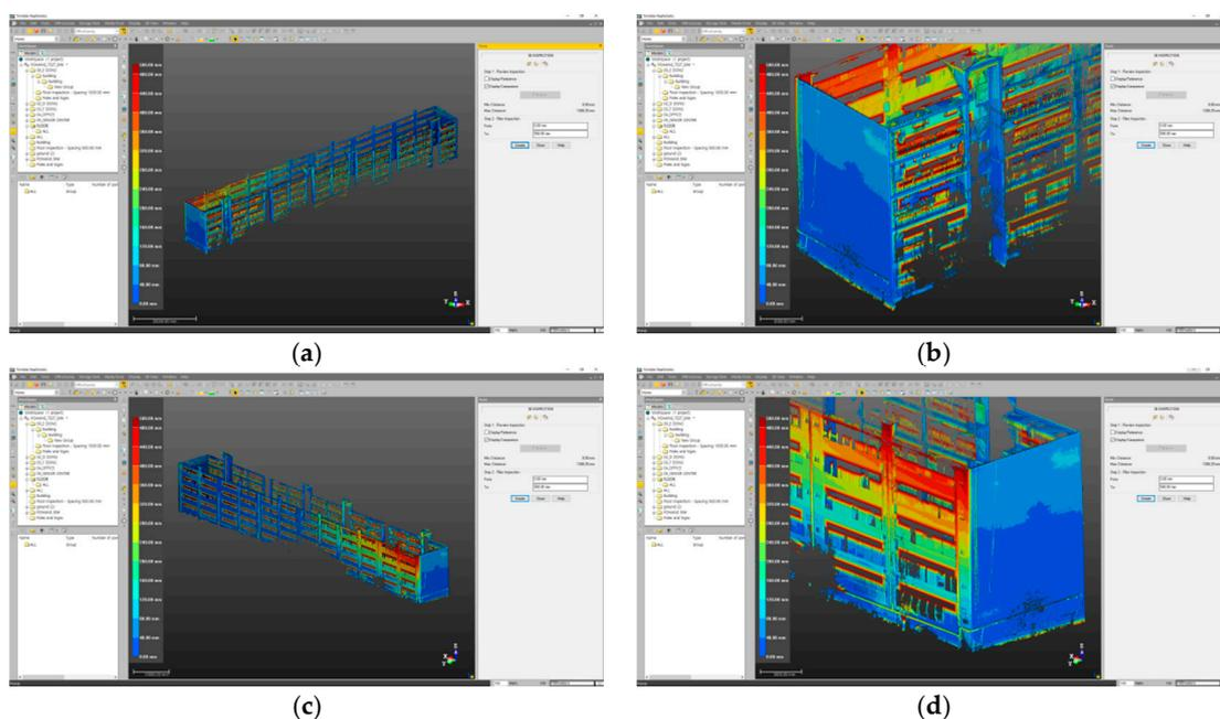
**Figure 7.** 3D inspection using the point cloud and BIM data. (a) Entire 3D inspection; (b) Front 3D inspection; (c) Rear 3D inspection; (d) Rear 3D inspection in detail.
