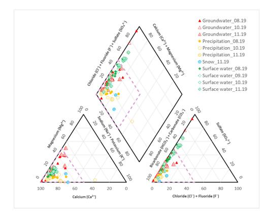
Figure 9. Piper diagram. The purple dotted line highlights the HCO<sub>3</sub>-Ca facies.
