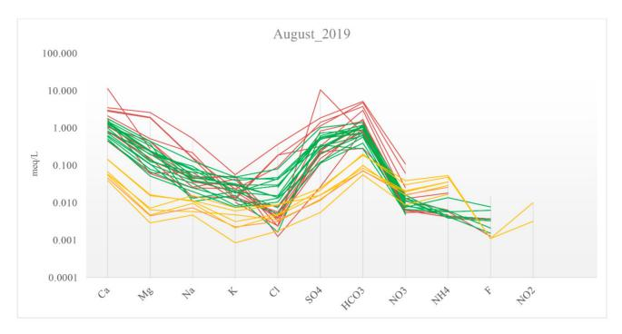
**Figure 8.** Schoeller diagram of waters sampled in August 2019. Green lines represent surface water, red lines represent groundwater and orange lines represent precipitation.
