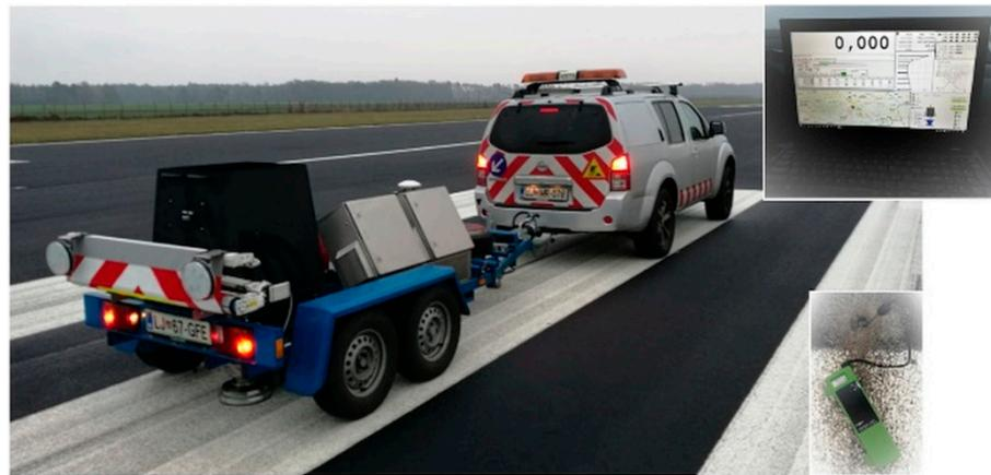
**Figure 3.** Using FWD equipment.
