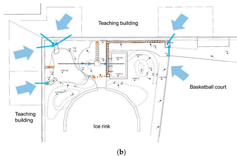
**Figure 5.** (a) Distribution of the water monitoring points at the BeiTou site and (b) the runoff collection route.
