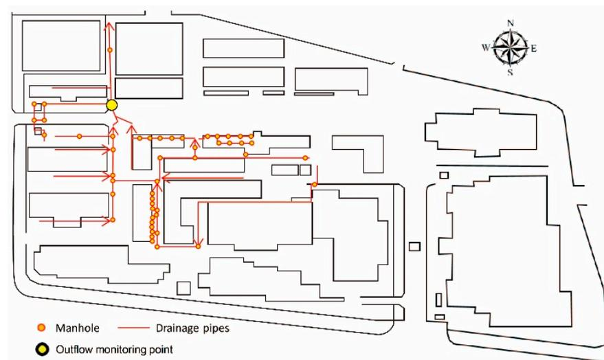
Figure 4. Drainage pipes at the Taipei Tech site and the outflow monitoring point.
