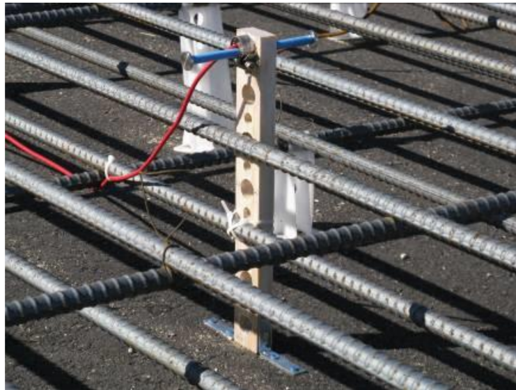
Figure 2. VWSG installed in the field.
