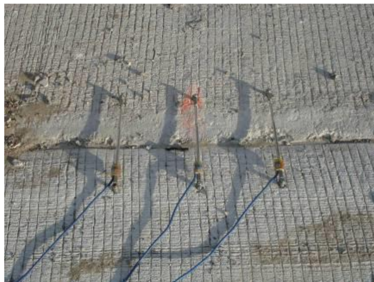
Figure 3. Crackmeters installed in each test section.
