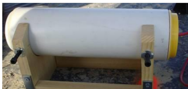
Figure 8. Nonstress cylinder installed in the field.
