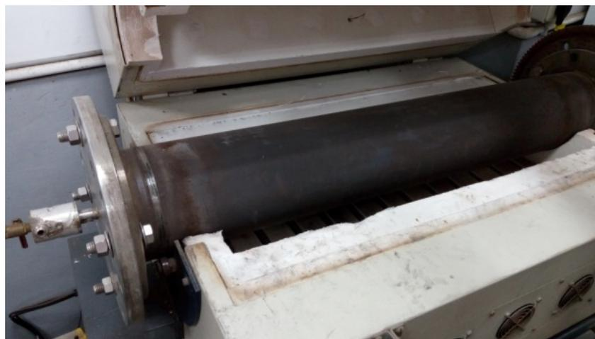
**Figure 7.** Photograph of prototype cyclone-type rotary kiln.
