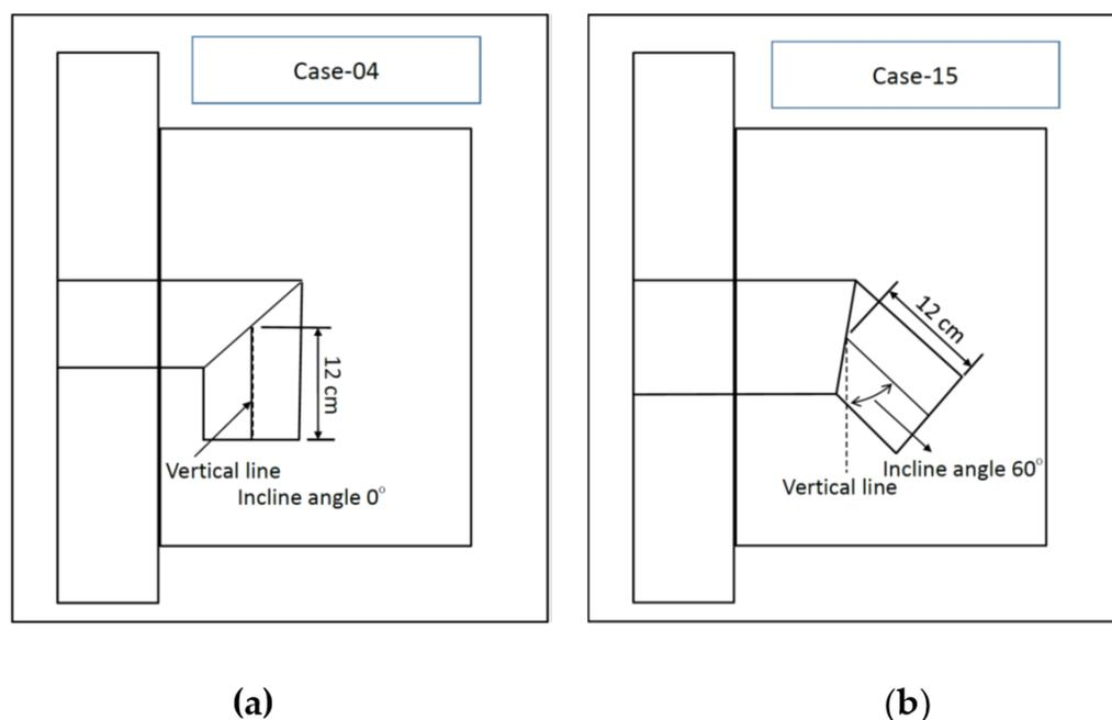
**Figure 4.** Geometry of inlet tube in: (a) 4th experiment; and (b) 15th experiment.
