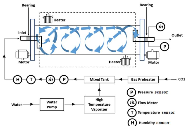
**Figure 2.** Flow field trajectory in the proposed cyclone-type rotary kiln reactor.
