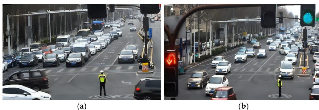
Figure 2. Problems with Variable direction Lanes: (a) Variable direction lane emptying, (b) Driver misses lane change.
