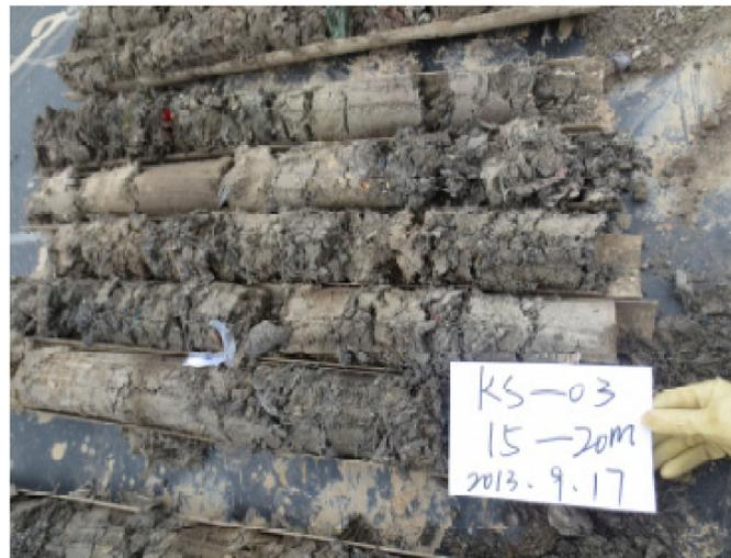
**Figure 2.** MSW drilled from the Jiangcungou landfill.
