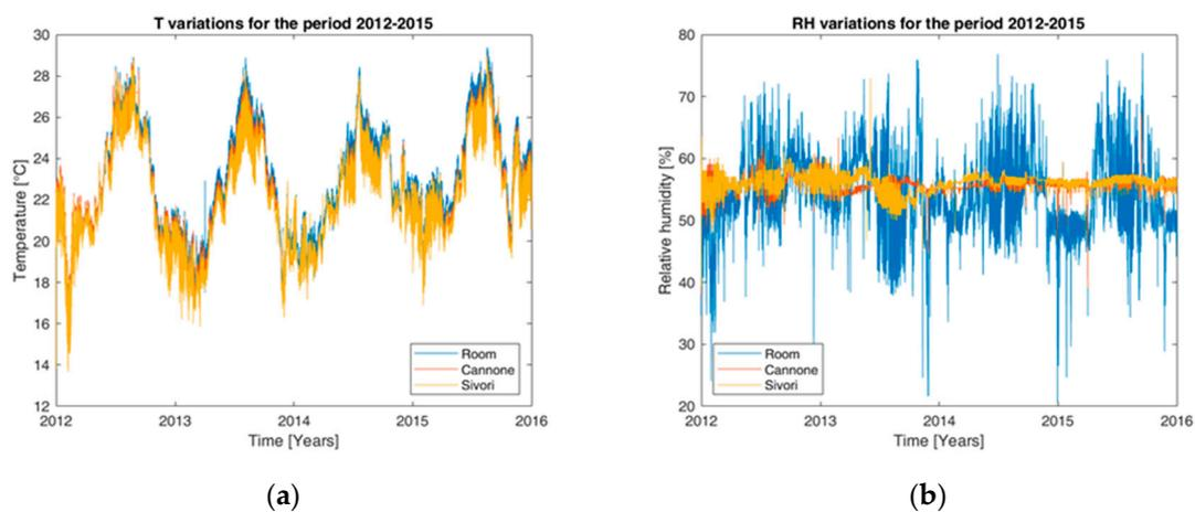
**Figure 2.** Variations of (a) temperature (T) and (b) relative humidity (RH) over time for the period January 2012–December 2015 for the three locations monitored: room, Cannone and Sivori display cases.
