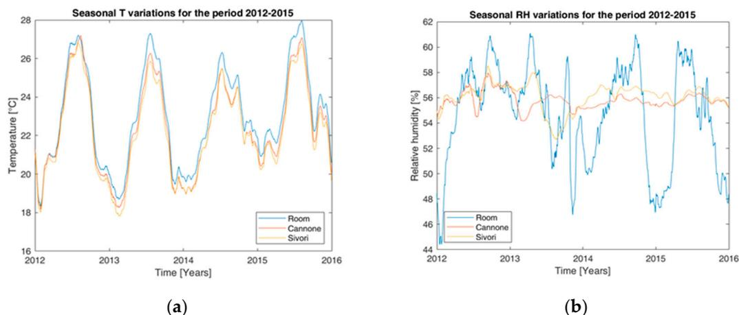
**Figure 3.** Seasonal variations of (a) T and (b) RH over time for the period January 2012–December 2015 for the three locations monitored: room, Cannone and Sivori display cases. The arrows indicate the installation of the control system on the two showcases (February 2013 on Cannone and September 2013 on Sivori).
