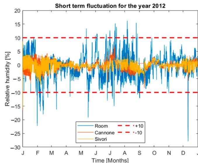
**Figure 4.** Short term fluctuation for the year 2012 for the three locations monitored: room, Cannone and Sivori display cases. The graph shows also the  $\pm 10\%$  fluctuations limits described by EN 15757:2010.
