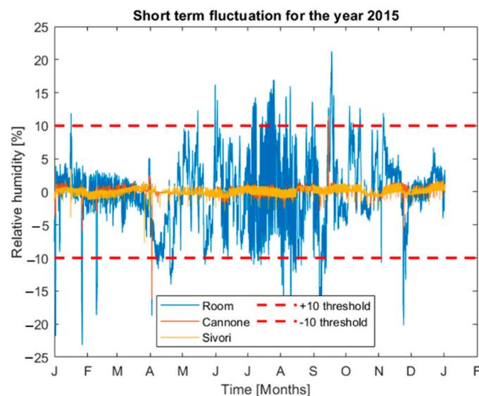
**Figure 5.** Short term fluctuation for the year 2015 for the three locations monitored: room, Cannone and Sivori display cases. The graph shows also the  $\pm 10\%$  fluctuation limits described by EN 15757:2010.
