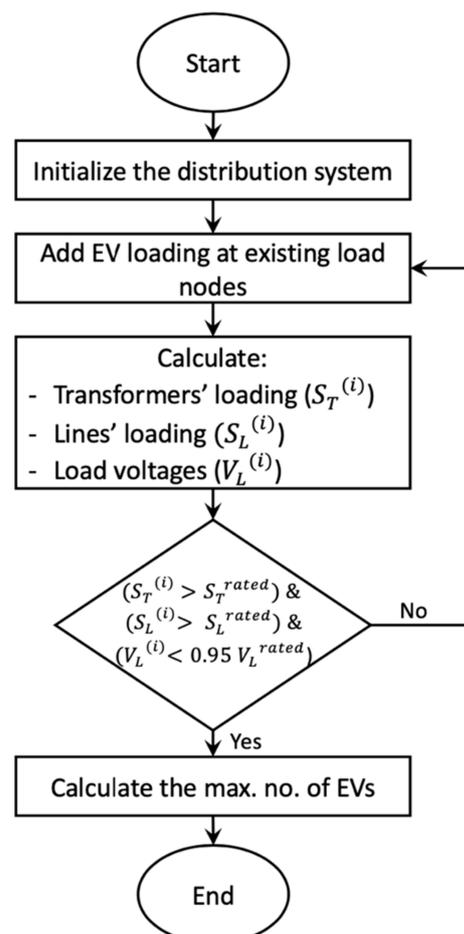
**Figure 4.** Flowchart for computation of the maximum number of EVs before reaching the three system violations.
