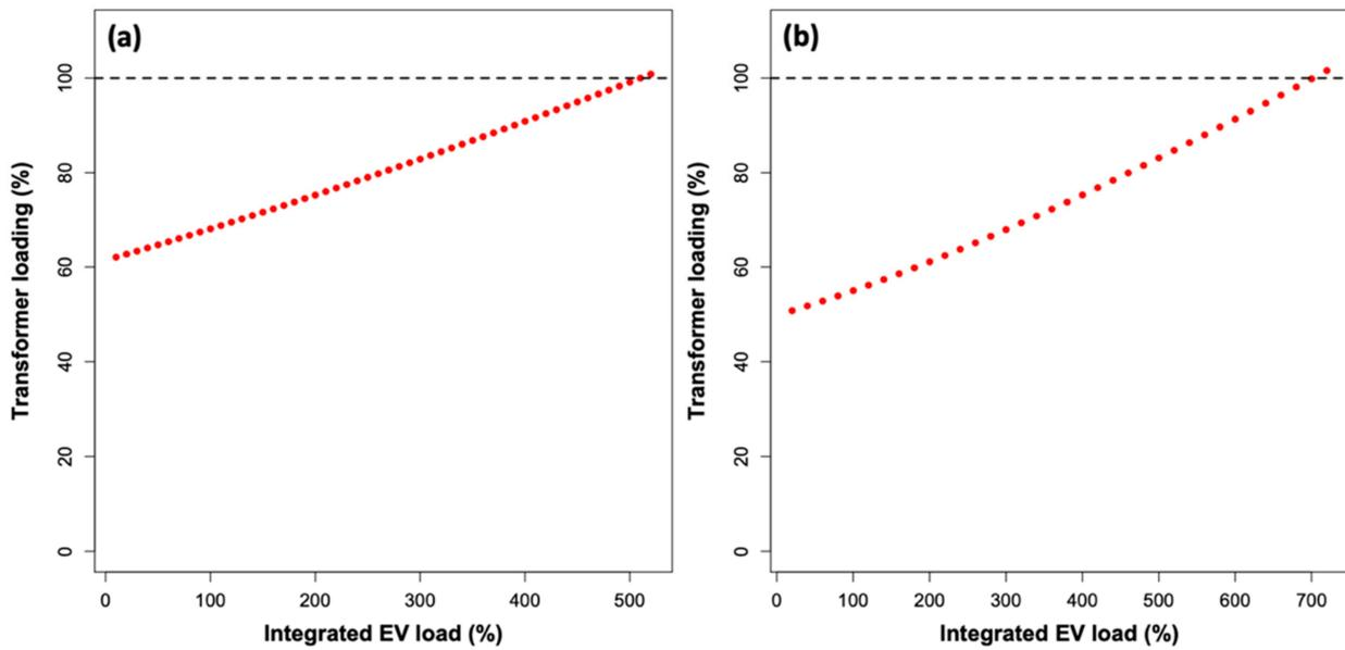
Figure A2. Scenario 2 at node 19: (a) Transformer loading at intermediate loading condition. (b) Transformer loading at light loading condition.
