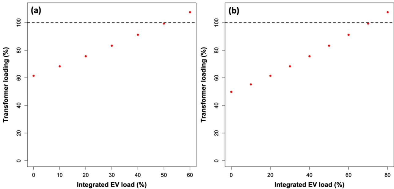
Figure A1. Scenario 1: (a) Transformer loading at intermediate loading condition. (b) Transformer loading at light loading condition.
