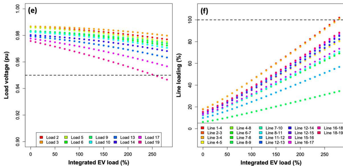
**Figure 5.** Scenario 1: (a) Load voltages at full loading condition. (b) Line loadings at full loading condition. (c) Load voltages at intermediate loading condition. (d) Line loadings at intermediate loading condition. (e) Load voltages at light loading condition. (f) Line loadings at light loading condition.
