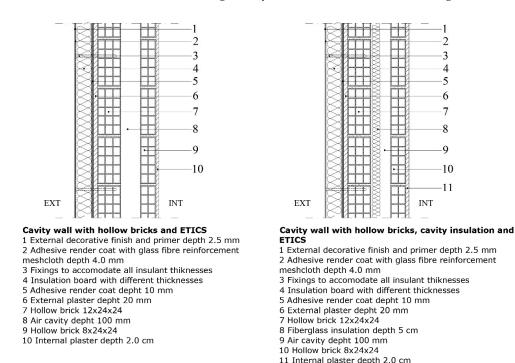
Figure 4. Reference walls insulated using ETICS (External Thermal Insulation Composite System).
