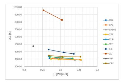
Figure 11. Life Cycle Cost (LCC) values as a function of U transmittance.
