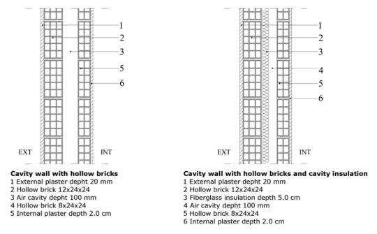
transmittance, U, up to a value equal to 0.53 W (m<sup>2</sup>K). Figure 2 shows the two reference stratigraphies mentioned.
