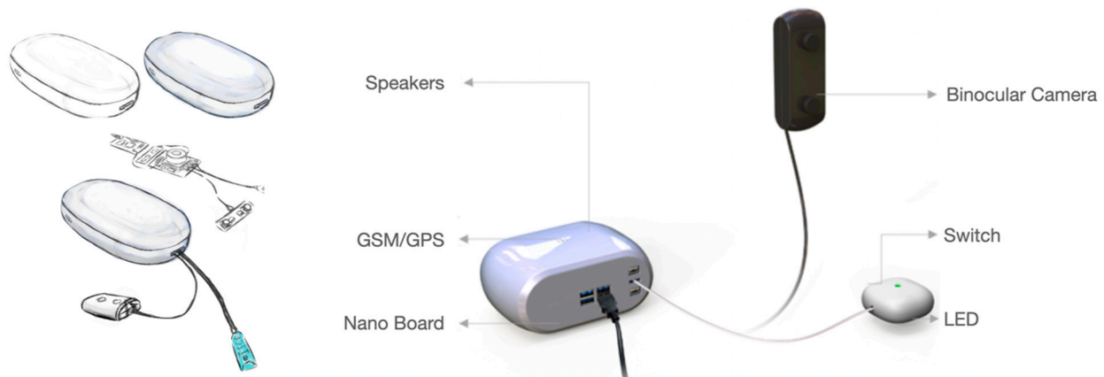
Figure 7. Left: a sketch of the components. Right: the schematics.
