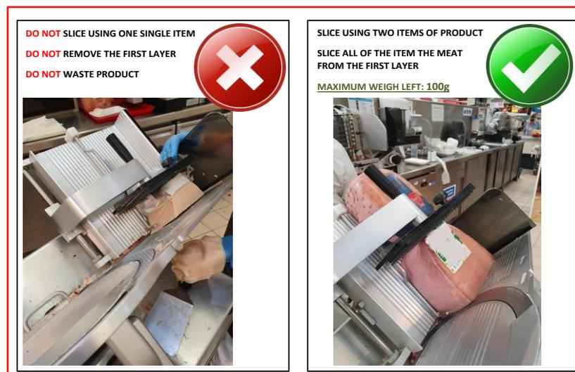
**Figure 4.** Visual standard for the “ham-cutting” operation created during the Kaizen event.
