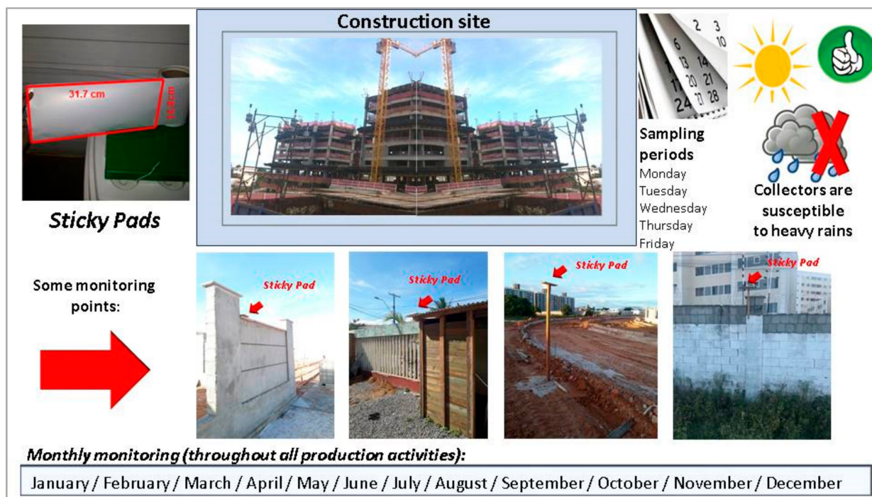
Figure 5. Scheme for monitoring sedimented particles on construction sites.
