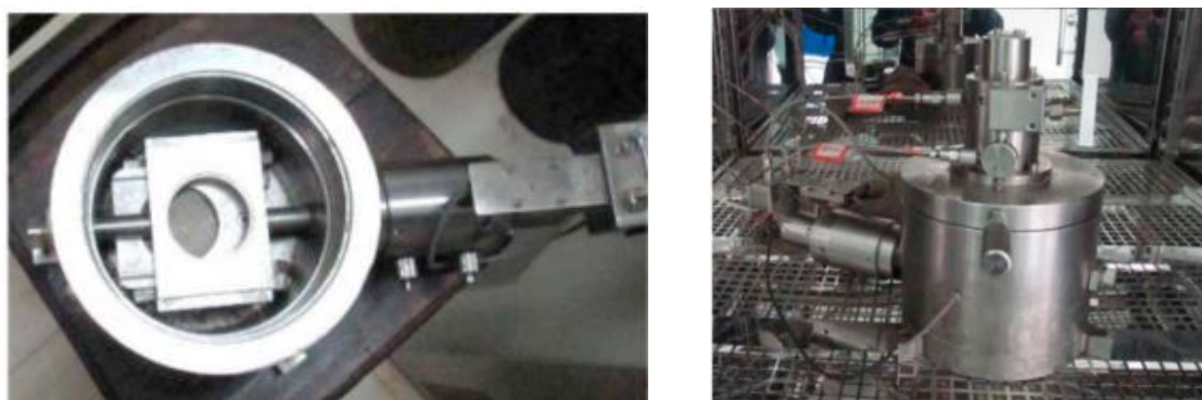
Figure 11. Diagram of the direct shear system [30].
