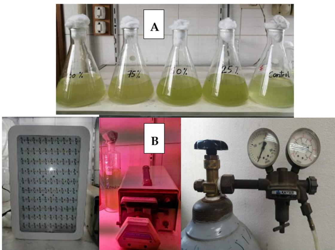
**Figure 3.** Biodesalination experimental system: (A) the system under control conditions, (B) the system under high light intensity and CO<sub>2</sub> conditions.
